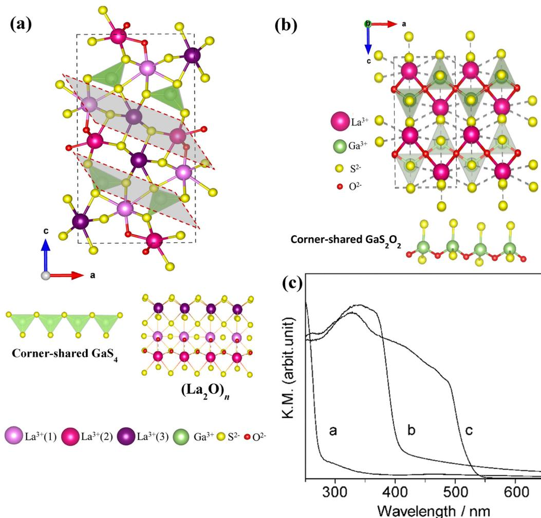
Fig. 7 Structural representation of (a)  $\text{La}_3\text{GaS}_5\text{O}$  ( $Pnma$  symmetry) and (b)  $\text{LaGaS}_2\text{O}$  ( $Pmca$  symmetry) and, highlighting the different layers between the two compounds; (c) shows diffuse reflectance data for (a)  $\text{LaGaO}_3$ , (b)  $\text{LaGaS}_2\text{O}$  and (c)  $\text{La}_3\text{GaS}_5\text{O}$ . Reprinted (adapted) with permission from *J. Phys. Chem. C*, 2008, **112**(31), 11978–11984. Copyright 2008 American Chemical Society.
