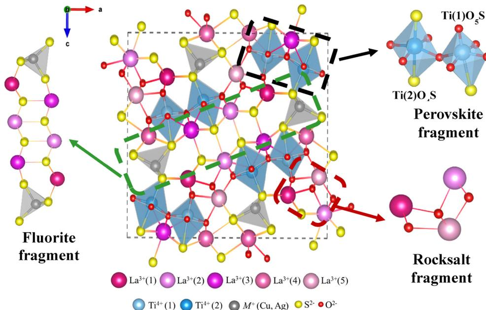
Fig. 8 Structural representation of (a)  $\text{La}_5\text{Ti}_2\text{MS}_5\text{O}_7$  ( $M = \text{Cu}, \text{Ag}$ ) oxysulfides ( $Pnma$  symmetry) highlighting the different building blocks within the structure.
