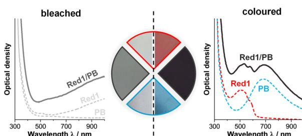
**Combining broadband absorbing electrochromic materials for hybrid grey-to-colourless flexible devices**
