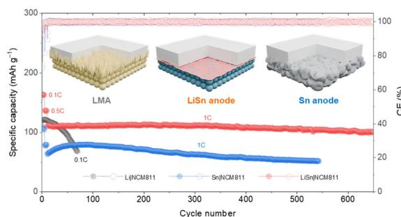
**An ultra-stable pre lithiated Sn anode for sulfide-based all-solid-state Li batteries**
