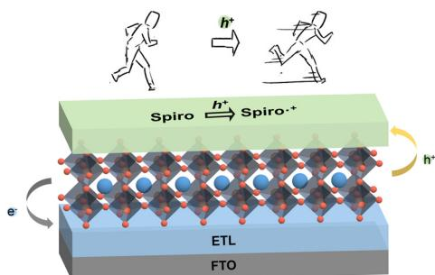
*In situ* fast oxidation of spiro-OMeTAD hole transport layers under ambient indoor lighting compatible with air-processed perovskite solar cells
