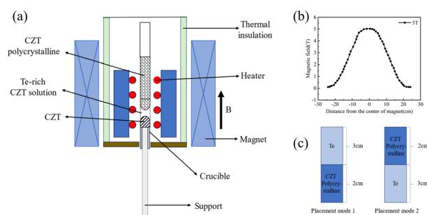
**Investigation of the diffusion and crystal growth of CdZnTe in Te solution using the traveling heater method under axial static magnetic field**
