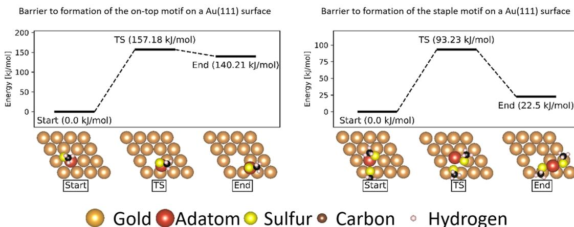
**Fig. 12** Energy barriers of formation of the on-top and staple motifs on a Au(111) surface. All energies are referenced to the starting state in the formation. The gold atoms are shown in brown, except for the gold adatom that is part of the thiolate motifs which is shown in red. The sulfur atoms are shown in yellow, the carbon atoms in black and the hydrogen atoms in pink.
