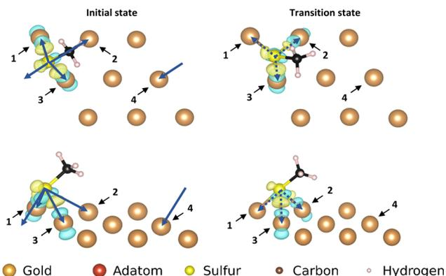
**Fig. 6** Electron density difference map (EDDM) for the 'free thiolate' motif; left: top and front view of the initial state of the movement, right: top and front view of the transition state of the movement. Only the top layer of the gold surface is shown for clarity. The arrows correspond with the pairs of atoms used in the corresponding COHP analysis.
