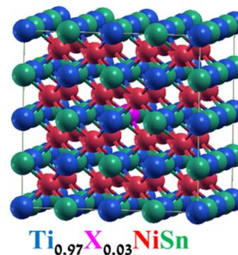
Fig. 1 96-atom supercell, replacing one Ti-atom (blue) with one atom of doping element (pink).
