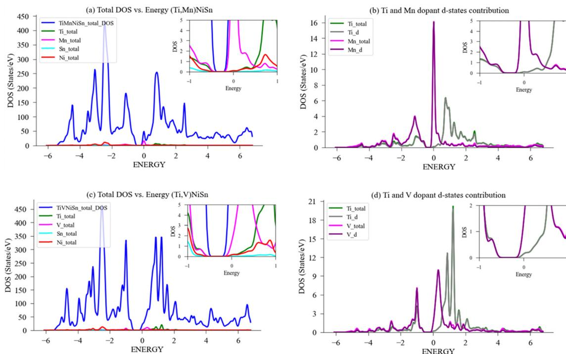
Fig. 8 DFT calculation of DOS for (Ti,X)NiSn with donor dopants. (a) Total and LDOS for compound with  $X = \text{Mn}$ ; (b) Ti, Mn PDOS-d contribution; (c) total and LDOS for compound with  $X = \text{V}$ ; (d) Ti, V PDOS-d contribution. A magnification of the area in the vicinity of Fermi energy,  $E_F$ , (set to zero) is shown in the inset.
