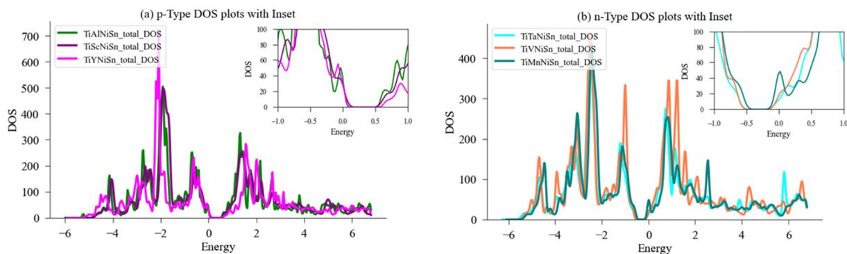
Fig. 6 Comparison of DOS for doped TiNiSn in the form of  $(\text{Ti}_{0.97}\text{X}_{0.03})\text{NiSn}$ . (a) Doped with acceptors ( $X = \text{Al}, \text{Sc}, \text{Y}$ ) forming p-type. (b) Doped with donors ( $X = \text{Ta}, \text{V}, \text{Mn}$ ) forming n-type. A magnification of the area in the vicinity of Fermi energy,  $E_F$ , (set to zero) is shown in the inset.
