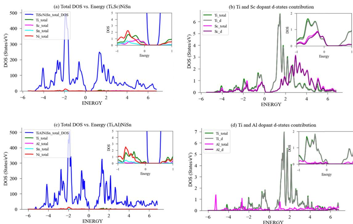
**Fig. 9** DFT calculation of DOS for (Ti,X)NiSn with acceptor dopants. (a) Total and LDOS for compound with X = Sc; (b) Ti, Sc PDOS-d contribution; (c) total and LDOS for compound with X = Al; (d) Ti, Al PDOS-d contribution. A magnification of the area in the vicinity of Fermi energy,  $E_F$ , (set to zero) is shown in the inset.
