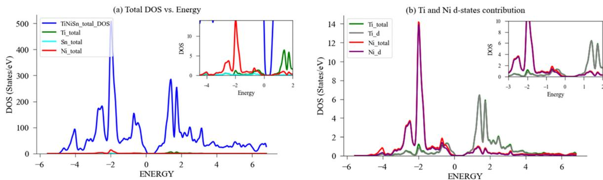
Fig. 7 DFT calculation of DOS for ideal TiNiSn. (a) Total and LDOS for 96-atom supercell; (b) Ti, Ni PDOS-d contribution. A magnification of the area in the vicinity of Fermi energy,  $E_F$ , (set to zero) is shown in the inset.
