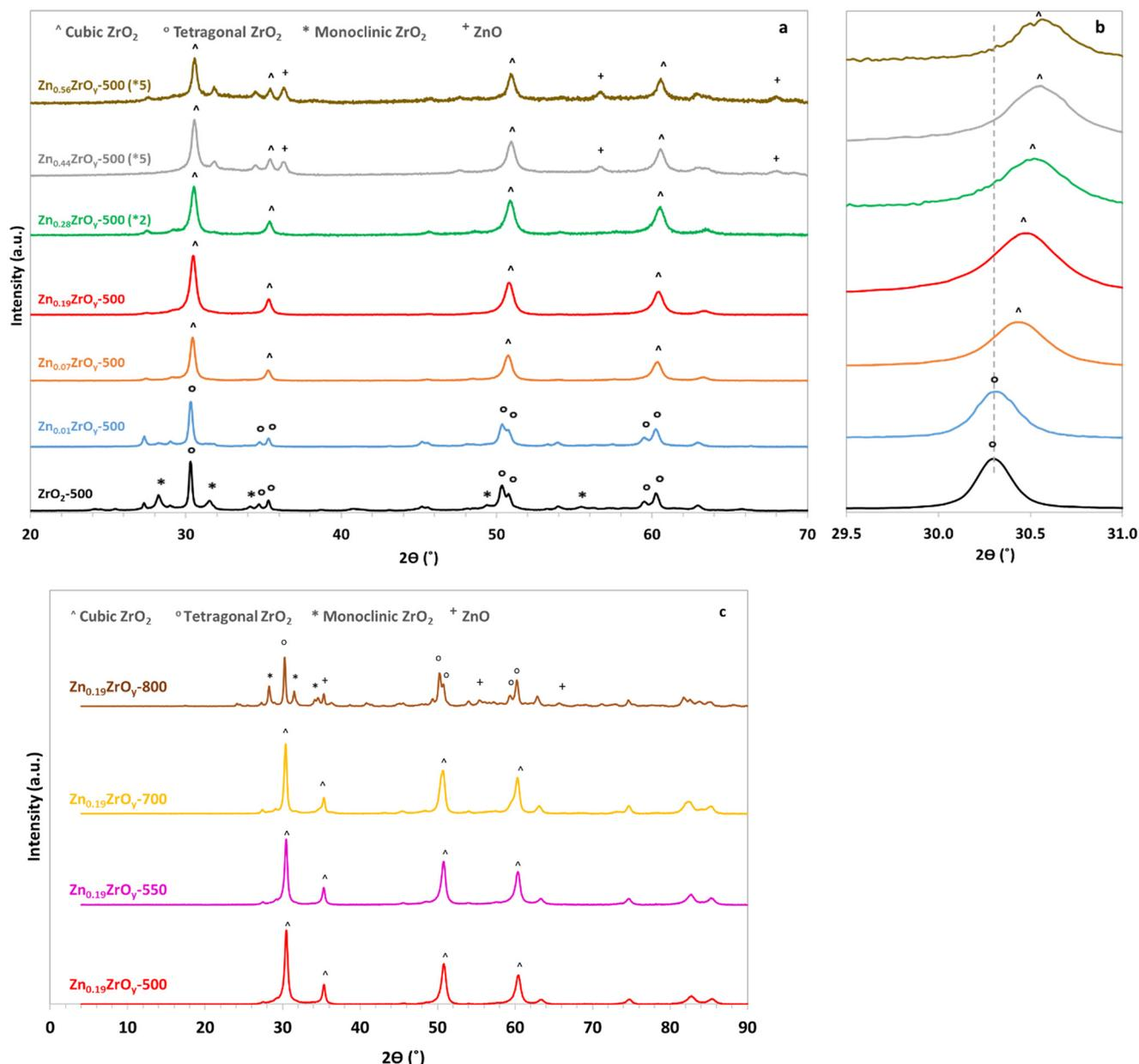
**Fig. 1** (a) XRD patterns of  $\text{Zn}_n\text{ZrO}_y\text{-500}$  catalysts, (b) enlarged XRD patterns of  $\text{Zn}_n\text{ZrO}_y\text{-500}$  catalysts in the  $2\theta$  range of  $29.5\text{--}31.0^\circ$ , and (c) XRD patterns of  $\text{Zn}_{0.19}\text{ZrO}_y\text{-}T$  calcined at 500, 550, 700, and 800 °C (m- $\text{ZrO}_2$ : PDF card 81.1314, t- $\text{ZrO}_2$ : PDF card 50-1089, c- $\text{ZrO}_2$ : PDF card 65-0461, and h- $\text{ZnO}$ : PDF card 05-0664).
