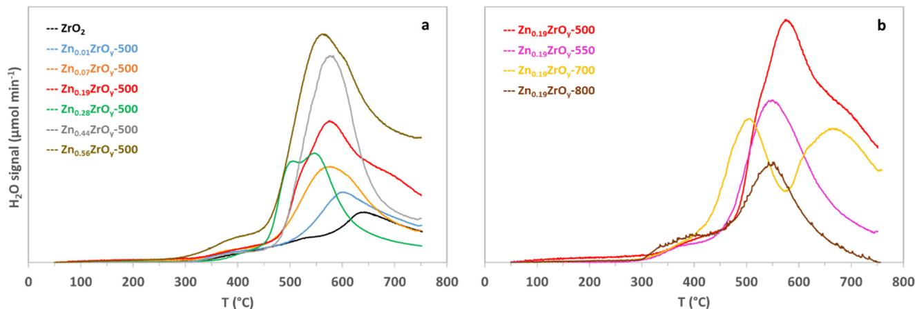
Fig. 4 Temperature-programmed H<sub>2</sub> reduction of (a) Zn<sub>x</sub>ZrO<sub>y</sub>-500 catalysts and (b) Zn<sub>0.19</sub>ZrO<sub>y</sub>-T calcined at 500, 550, 700, and 800 °C.
