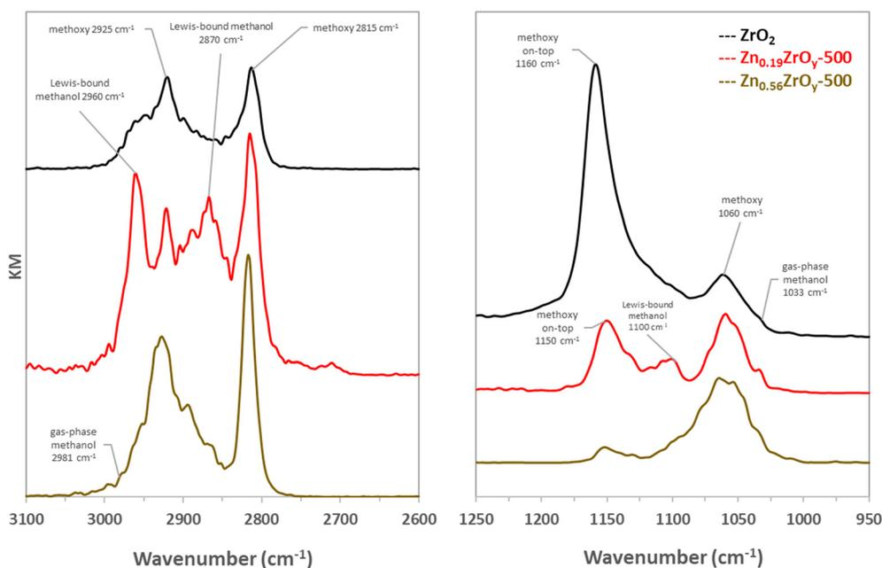
Fig. 7 DRIFT spectra of methanol adsorption at 200 °C and 10 bar on  $ZrO_2$ ,  $Zn_{0.19}ZrO_y$ -500, and  $Zn_{0.56}ZrO_y$ -500 (the spectra were recorded after evacuation of physically adsorbed species under a flow of 130  $ml\ min^{-1}$  Ar).
