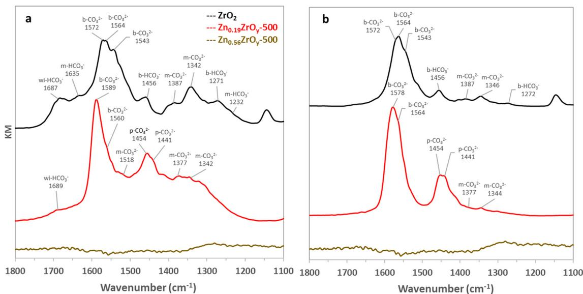
Fig. 6 DRIFT spectra of (a)  $\text{CO}_2$  adsorption at 325 °C and 10 bar on  $\text{ZrO}_2$ ,  $\text{Zn}_{0.19}\text{ZrO}_y$ -500, and  $\text{Zn}_{0.56}\text{ZrO}_y$ -500 after 40 minutes under 2  $\text{ml min}^{-1}$   $\text{CO}_2$  and 16  $\text{ml min}^{-1}$  Ar and (b) after 40 minutes evacuation at 325 °C and 10 bar under 16  $\text{ml min}^{-1}$  Ar (m: monodentate, b: bidentate, wi: weakly interacting, and p: polydentate species).
