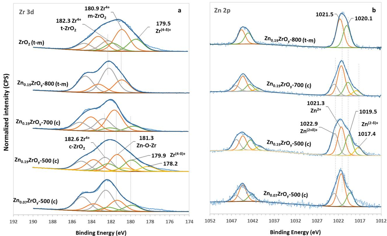
Fig. 3 XPS spectra of (a) Zr 3d in  $\text{ZrO}_2$ ,  $\text{Zn}_{0.07}\text{ZrO}_y\text{-}500$ ,  $\text{Zn}_{0.19}\text{ZrO}_y\text{-}500$ ,  $\text{Zn}_{0.19}\text{ZrO}_y\text{-}700$ , and  $\text{Zn}_{0.19}\text{ZrO}_y\text{-}800$  and (b) Zn 2p in  $\text{Zn}_{0.07}\text{ZrO}_y\text{-}500$ ,  $\text{Zn}_{0.19}\text{ZrO}_y\text{-}500$ ,  $\text{Zn}_{0.19}\text{ZrO}_y\text{-}700$ , and  $\text{Zn}_{0.19}\text{ZrO}_y\text{-}800$ .
