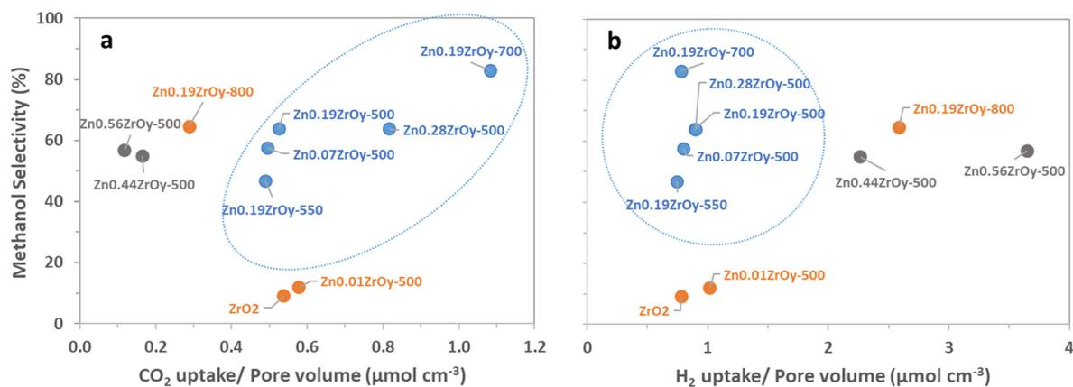
**Fig. 10** Effect of pore-volume normalized (a) CO<sub>2</sub> uptake and (b) H<sub>2</sub> uptake on methanol selectivity at 350 °C, 45 bar, H<sub>2</sub>:CO<sub>2</sub>:Ar = 3:1:1, and GHSV = 21 000 Nml g<sub>cat</sub><sup>-1</sup> h<sup>-1</sup> (blue colour: pure cubic-phase, grey colour: cubic-phase + h-ZnO, and orange colour: the rest of the samples).
