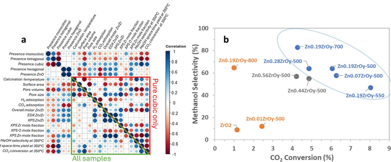
**Fig. 9** (a) Surface property correlations and CTM catalysis within all samples and (b) methanol selectivity versus CO<sub>2</sub> conversion at 350 °C, 45 bar, H<sub>2</sub>:CO<sub>2</sub>:Ar = 3:1:1, and GHSV = 21 000 Nml g<sub>cat</sub><sup>-1</sup> h<sup>-1</sup> (blue colour: pure cubic-phase, grey colour: cubic-phase + h-ZnO, and orange colour: the rest of the samples).
