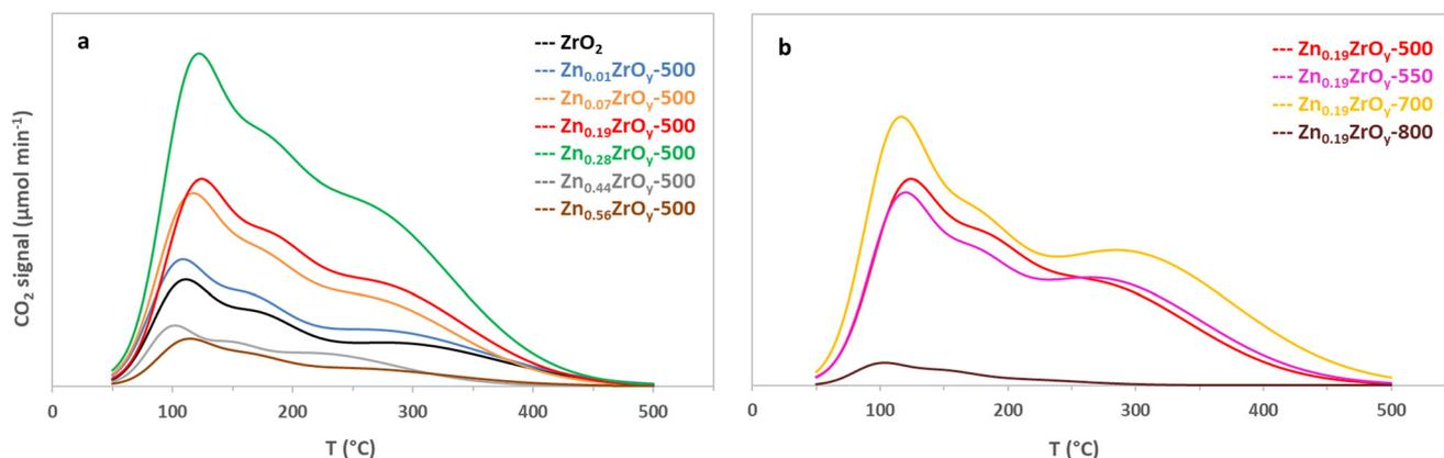
Fig. 5 Temperature-programmed CO<sub>2</sub> desorption of (a) Zn<sub>x</sub>ZrO<sub>y</sub>-500 catalysts and (b) Zn<sub>0.19</sub>ZrO<sub>y</sub>-T calcined at 500, 550, 700, and 800 °C.
