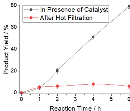
**Fig. 3** Product yield of 5-phenyltetrazole as determined by <sup>1</sup>H-NMR in presence of polystyrene-bound AlCl<sub>3</sub> as heterogeneous catalyst (black) or after hot filtration after 1 hour (red).
