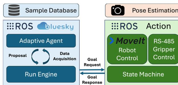
**Fig. 2** Architecture schematic for robotic beamline scientist. Primarily a client-server architecture, the approach to integrating the robotic beamline scientist into the experiment orchestration with *Bluesky* leveraged a sample database, ROS2 Action and pose estimation service. The *Bluesky* RunEngine orchestrates the overall experiment in a closed loop, where an adaptive agent provides recommendations for the next experiment and the Action server orchestrates the robotic subsystem.
