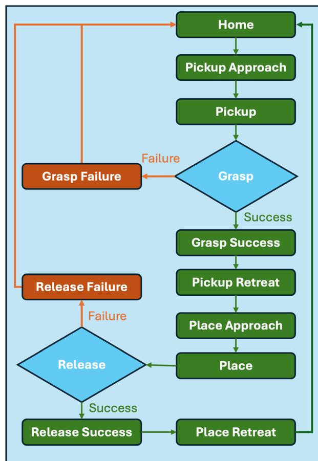
Fig. 4 The robot Action progression used a finite state machine to track progress. This FSM provided dynamic feedback to the *Bluesky* RunEngine for progress updates and synchronization management.
