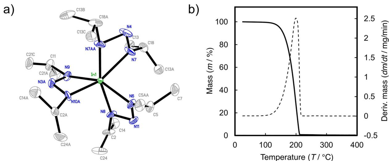
**Fig. 2** (a) X-ray crystal structure of In(triaz)<sub>3</sub> with thermal ellipsoids at the 50% probability level. All hydrogen atoms were removed for clarity. (b) TGA of In(triaz)<sub>3</sub> showing near ideal single step volatilisation with negligible residue mass. Images are reprinted from O'Brien *et al.*<sup>35</sup> under a CC-BY license.
