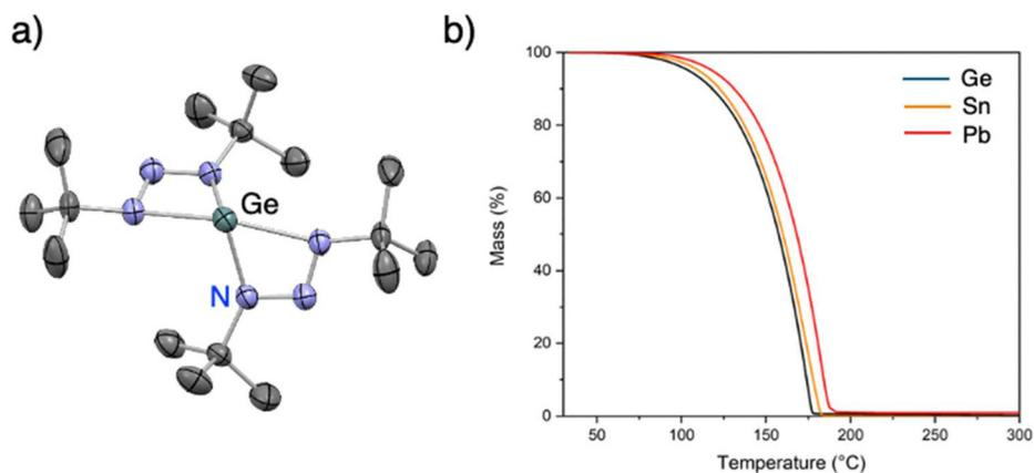
**Fig. 7** (a) X-ray crystal structure of the Ge triazenide precursor with thermal ellipsoids at the 50% probability level. All hydrogen atoms were removed for clarity. (b) The TGA graphs of Ge, Sn and Pb triazenides. Reprinted from Samii *et al.*<sup>44</sup> under a CC-BY license.
