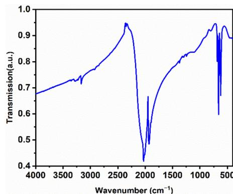
Fig. 9 FT-IR spectrum of  $La_2(CN_2)_3$ .
