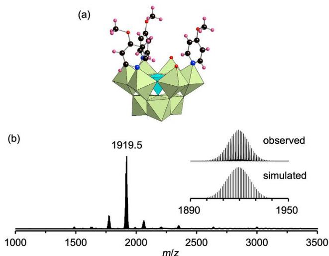
**Fig. 3** (a) Crystal structure of the anionic component of **I<sub>As</sub>**. (b) ESI-mass spectrum of **I<sub>As</sub>** in acetonitrile. Inset: Enlarged spectrum (top) and simulated pattern of [TBA<sub>2</sub>AsMo<sub>9</sub>O<sub>31</sub>]<sup>-</sup> ( $m/z$ : 1919.5, bottom). Light green octahedra and the light blue tetrahedron represent [MoO<sub>6</sub>] and [AsO<sub>4</sub>], respectively. Red, black, pink, and blue spheres denote O, C, H, and N atoms, respectively.
