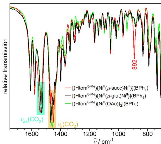
**Fig. 1** FTIR spectra of  $[[\text{(Htom}^{6\text{-Me}}\text{Ni}^{\text{II}}(\mu\text{-succ})\text{Ni}^{\text{II}})](\text{BPh}_4)]$ ,  $[[\text{(Htom}^{6\text{-Me}}\text{Ni}^{\text{II}}(\mu\text{-glut})\text{Ni}^{\text{II}})](\text{BPh}_4)]$ , and  $[[\text{(Htom}^{6\text{-Me}}\text{Ni}^{\text{II}}(\text{OAc}))_2](\text{BPh}_4)]^7$  for comparison.
