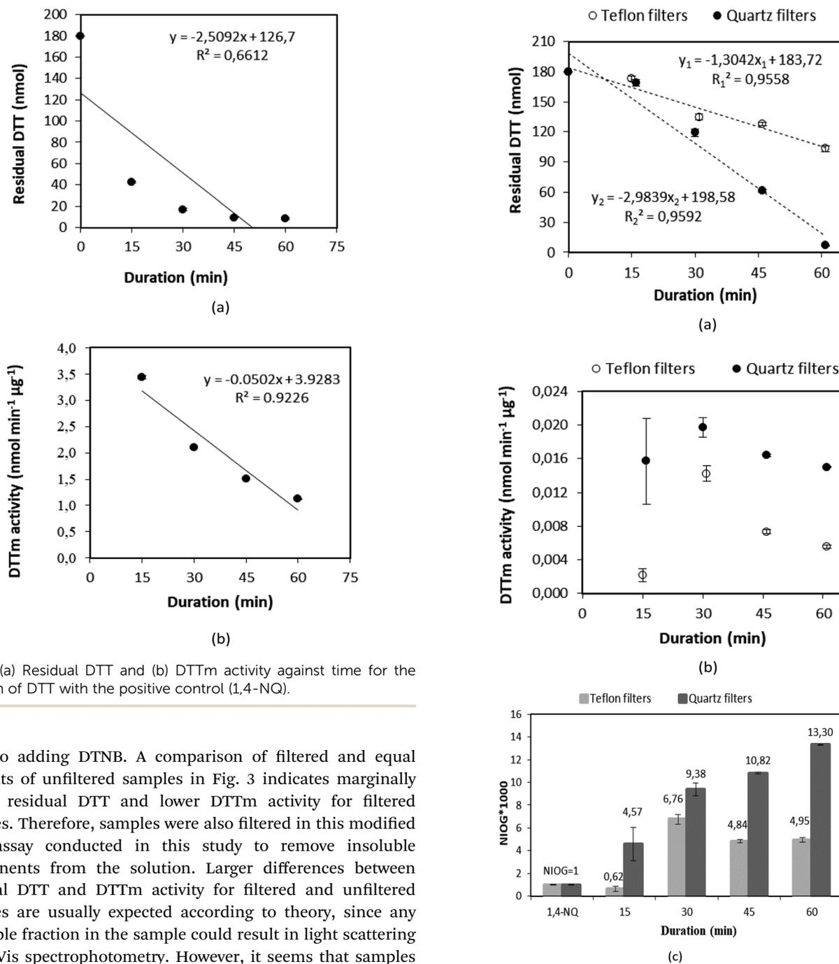
Fig. 4 (a) Residual DTT and (b) DTTm activity against time for the reaction of DTT with the positive control (1,4-NQ).
