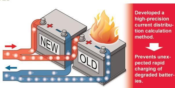
**Current distribution simulation of parallel-connected modules using degraded lithium-ion battery cells**
