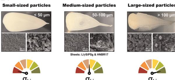
**Effect of particle size on the slurry-based processability and conductivity of  $t\text{-Li}_2\text{SiPS}_8$**
