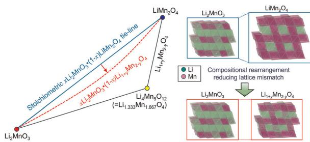
**Intrinsic mechanisms for structural coherency and electrochemical excellence in layered-spinel Li–Mn–O cathodes**
