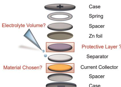
**Small changes, big gains: standardizing non-electrode coin cell components in aqueous zinc battery research**
