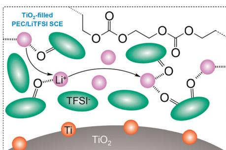
**Molecular dynamics of the coordination effect and ionic transport in  $\text{TiO}_2$ -filled poly(ethylene carbonate)-based electrolytes**
