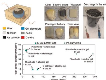
**Small-scale, long-duration, and biodegradable zinc–air batteries**
