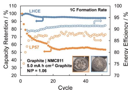
**Enabling fast formation for lithium-ion batteries with a localized high-concentration electrolyte**
