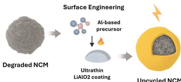
**Direct upcycling of degraded NCM via low-temperature surface engineering for high performance lithium-ion batteries**
