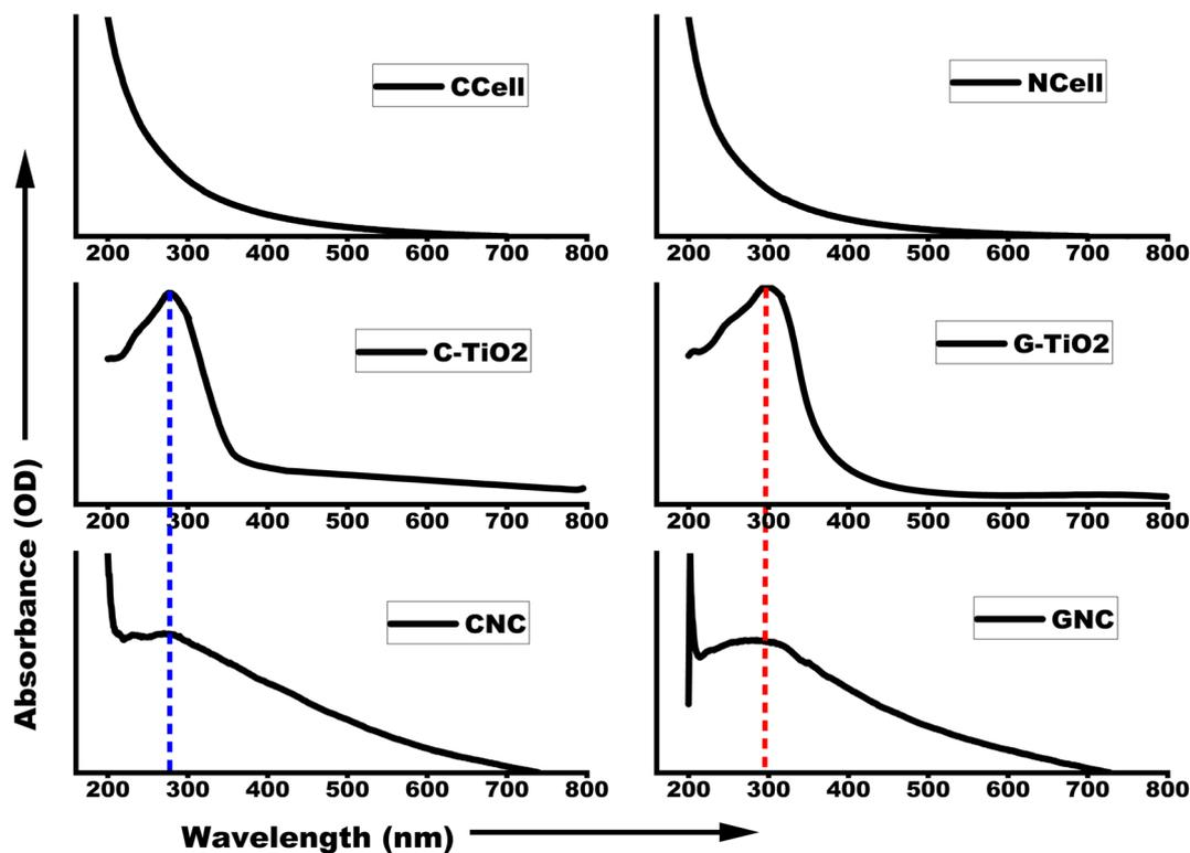
Fig. 2 Absorption profile of cotton extracted cellulose (CCell), nanocrystalline cellulose (NCell), C-TiO<sub>2</sub> (chemical TiO<sub>2</sub>), G-TiO<sub>2</sub> (green synthesized TiO<sub>2</sub>), CNC (NCell : C-TiO<sub>2</sub> nanocomposite) and GNC (NCell : G-TiO<sub>2</sub> nanocomposite) obtained from UV-visible spectroscopy.
