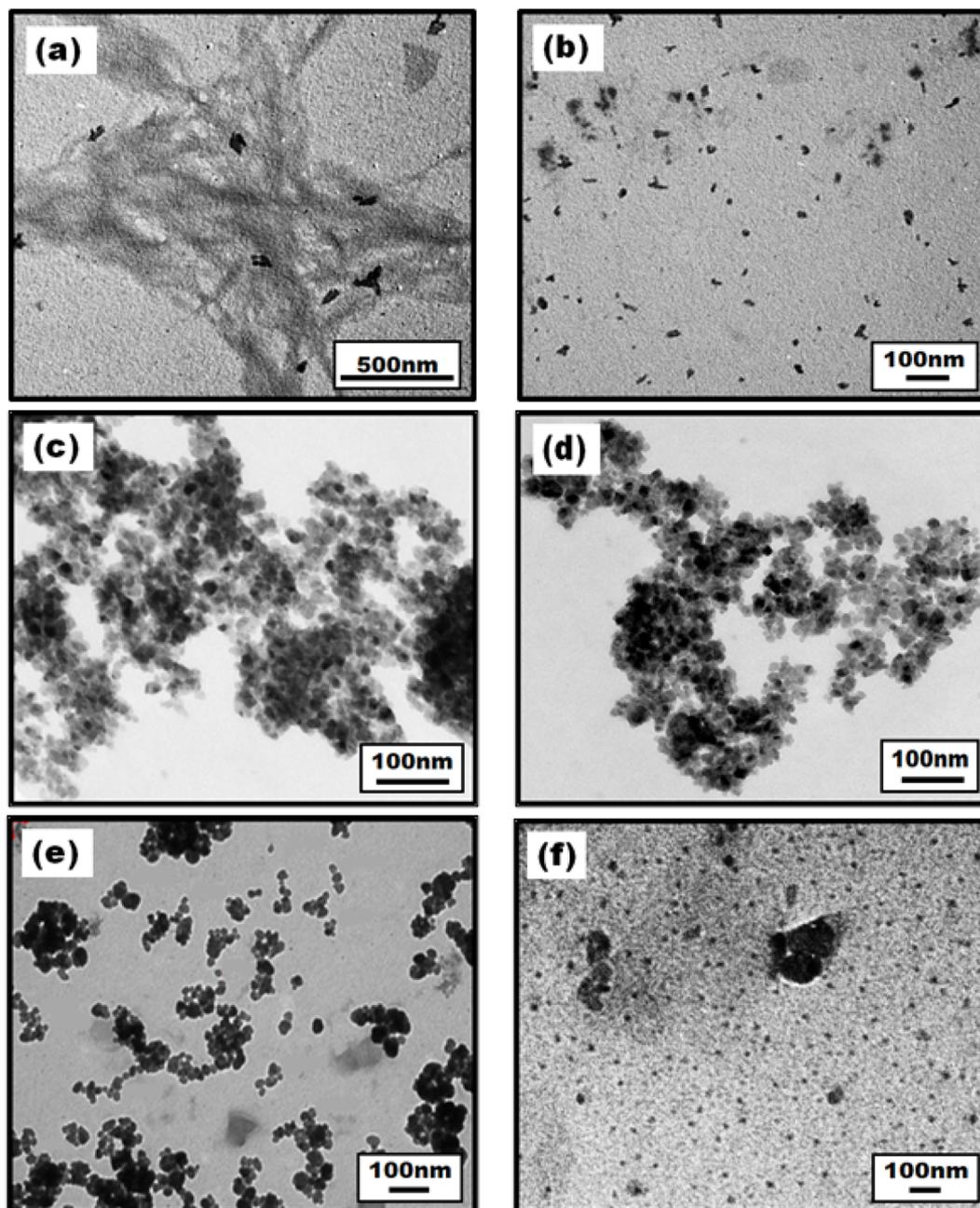
Fig. 3 Images recorded using a transmission electron microscope (TEM) for (a) cotton-extracted cellulose, (b) nanocrystalline cellulose, (c) chemical  $\text{TiO}_2$ , (d) green synthesized  $\text{TiO}_2$ , (e) CNC (NCell : C- $\text{TiO}_2$  nanocomposite) and (f) GNC (NCell : G- $\text{TiO}_2$  nanocomposite).
