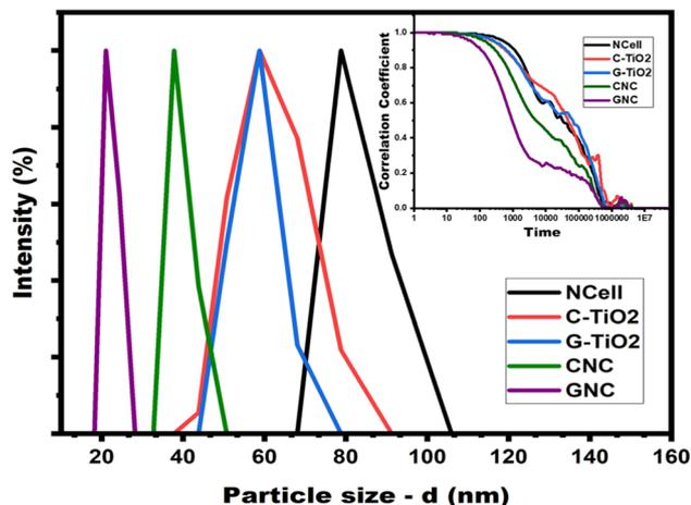
Fig. 4 DLS spectra showing the particle size distribution of (a) nanocrystalline cellulose (NCell), (b) chemical  $\text{TiO}_2$  (C- $\text{TiO}_2$ ), (c) green synthesized  $\text{TiO}_2$  (G- $\text{TiO}_2$ ), (d) CNC (NCell : C- $\text{TiO}_2$  nanocomposite) and (e) GNC (NCell : G- $\text{TiO}_2$  nanocomposite); inset showing the correlation coefficient versus time plot of all the samples.
