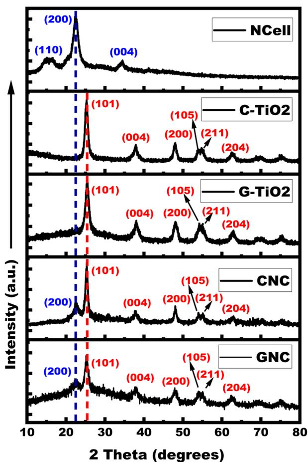
Fig. 1 X-ray diffraction pattern of nanocrystalline cellulose (NCell), C-TiO<sub>2</sub> (chemical TiO<sub>2</sub>), G-TiO<sub>2</sub> (green synthesized TiO<sub>2</sub>), CNC (NCell : C-TiO<sub>2</sub> nanocomposite) and GNC (NCell : G-TiO<sub>2</sub> nanocomposite).
