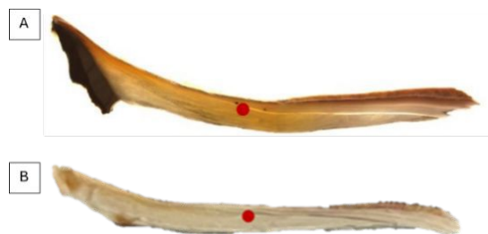
Figure 3 : (A) Scallop sample from non-contaminated Bradda area and (B) scallop sample from metal contaminated Laxey area, longitudinal section view. The region of interest is marked with a red circle.
