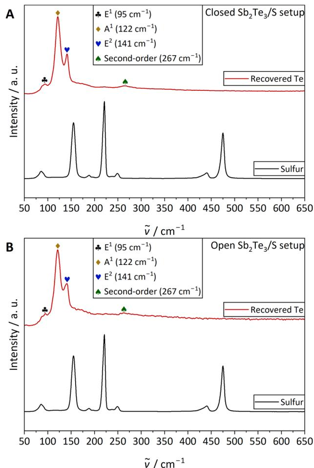
**Fig. 9** Raman spectra of tellurium recovered in (A) the best closed and (B) the best open  $\text{Sb}_2\text{Te}_3/\text{S}$  experimental setup. A reference measurement of sulfur is also shown, and the specific Raman modes of tellurium are marked.
