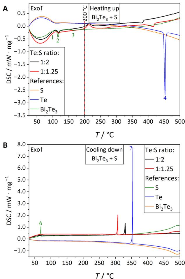
**Fig. 2** DSC cycles (A: heating, B: cooling) of mixtures of bismuth telluride and sulfur for two different Te:S molar ratios (black: 1:2, red: 1:1.25) and for sulfur (green), tellurium (blue) and bismuth telluride (orange) as references. Additionally, in (A), the onset value of the redox reaction is marked with red and black lines.
