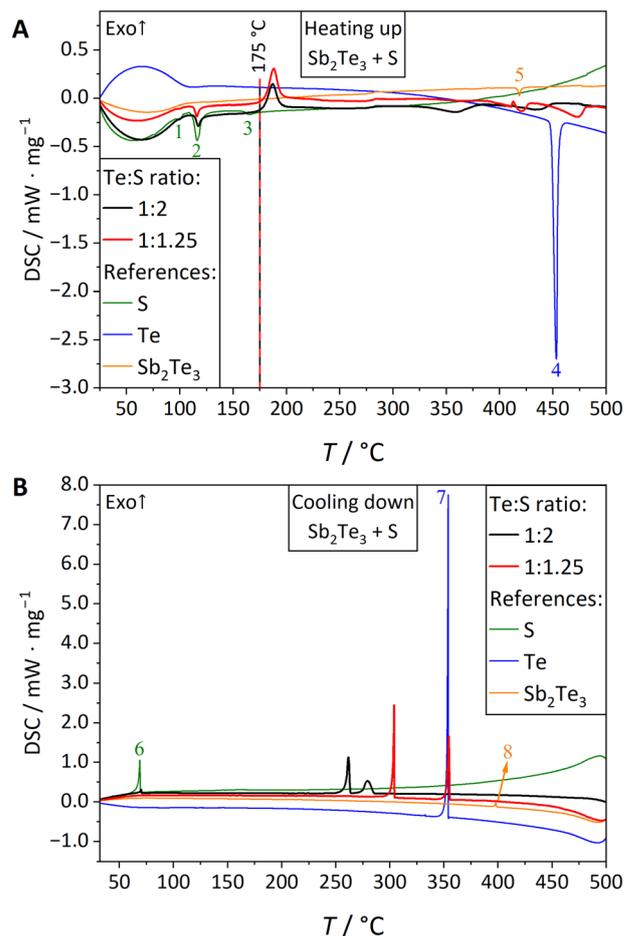
**Fig. 3** DSC cycles (A: heating, B: cooling) of mixtures of antimony telluride and sulfur for two different Te:S molar ratios (black: 1:2, red: 1:1.25) and for sulfur (green), tellurium (blue) and antimony telluride (orange) as references. Additionally, in (A), the onset value of the redox reaction is marked with red and black lines.
