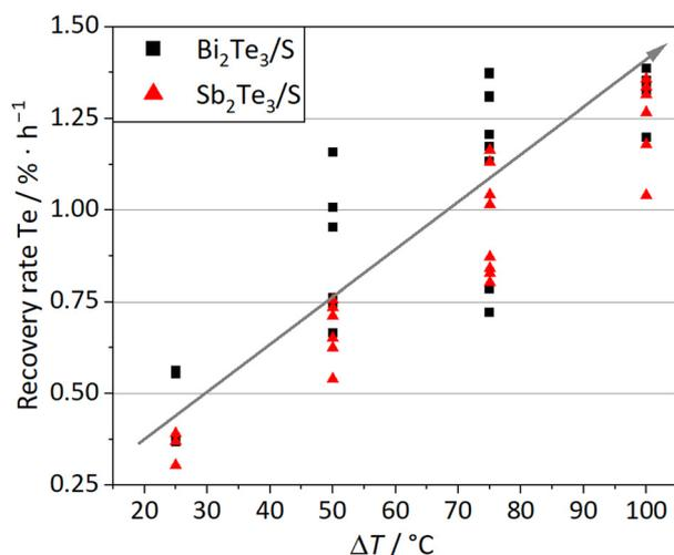
**Fig. 5** Recovery rate of Te in relation to the temperature difference  $\Delta T$  between the source and sink for the  $\text{Bi}_2\text{Te}_3/\text{S}$  (black squares) and  $\text{Sb}_2\text{Te}_3/\text{S}$  (red triangles) systems.
