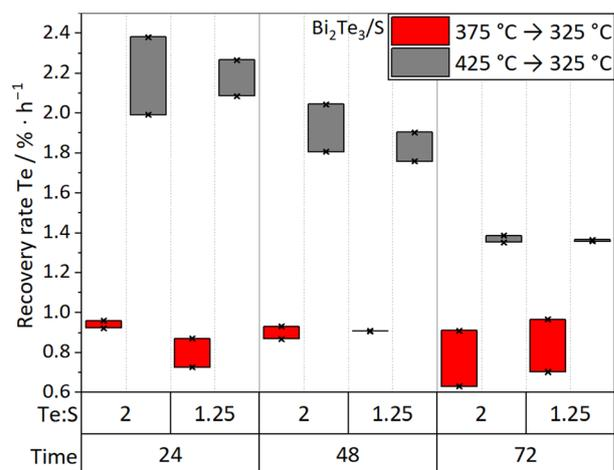
**Fig. 6** Recovery rates of Te for the  $\text{Bi}_2\text{Te}_3/\text{S}$  system in relation to two different Te : S molar ratios (1 : 2, 1 : 1.25) at two different temperature gradients (red boxes: 375 °C → 325 °C, grey boxes: 425 °C → 325 °C) and a reaction time of 24 h, 48 h or 72 h. The exact transport rates for each ampoule are marked with a black cross.
