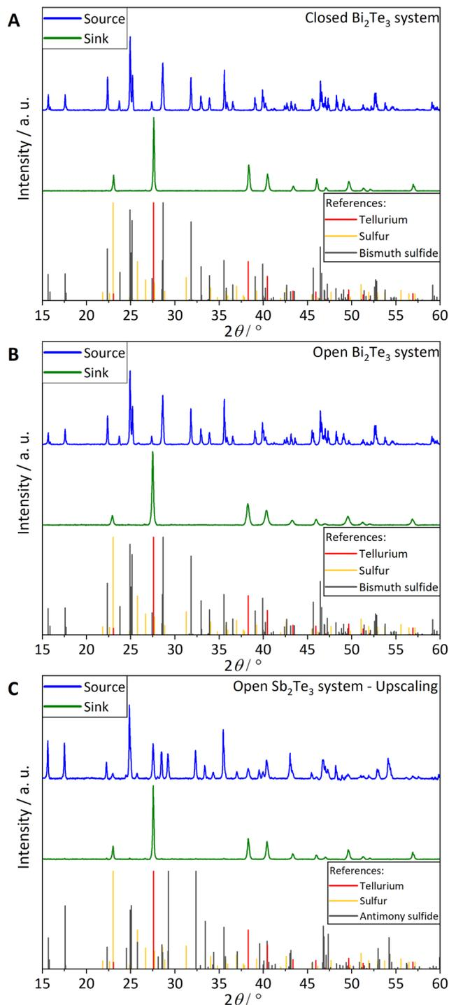
**Fig. 8** PXRD data of the source (blue diffractogram) and sink (green diffractogram) products of (A) the best closed and (B) the best open  $\text{Bi}_2\text{Te}_3/\text{S}$  experimental setup and (C) the  $\text{Sb}_2\text{Te}_3/\text{S}$  upscaling setup. Additionally, references for tellurium,<sup>33</sup> sulfur,<sup>34</sup> bismuth sulfide<sup>35</sup> and antimony sulfide<sup>36</sup> are shown.
