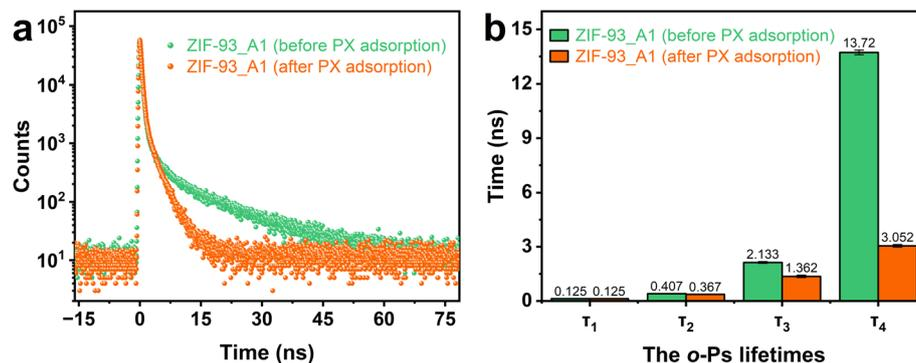
Fig. 9 (a) Peak-normalized positron lifetime spectrum and (b) *o*-Ps lifetimes for ZIF-93\_A1 before and after adsorption of *p*-xylene.
