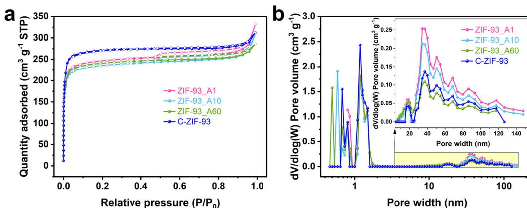
Fig. 4 (a) N<sub>2</sub> adsorption–desorption isotherms and (b) pore size distributions of ZIF-93\_A1 and C-ZIF-93 samples.
