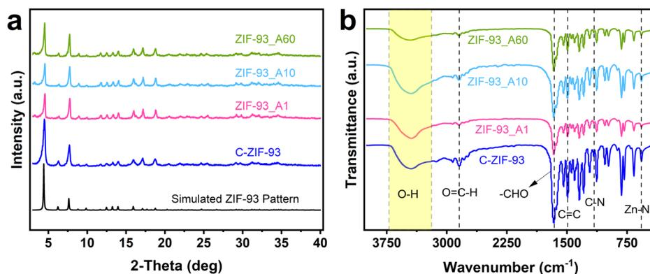
Fig. 1 (a) Powder XRD patterns of ZIF-93\_A*t* (*t* = 1, 10, 60) and C-ZIF-93 samples and simulated XRD pattern of ZIF-93. (b) FT-IR spectra of the as-synthesized ZIF-93\_A*t* (*t* = 1, 10, 60) and C-ZIF-93.
