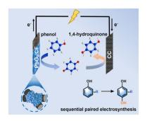
Membrane-free sequential paired electrosynthesis of 1,4-hydroquinone from phenol over a selfsupported electrocatalytic electrode
