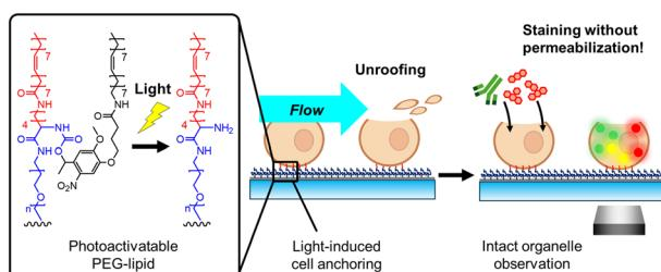
**Microfluidic cell unroofing for the *in situ* molecular analysis of organelles without membrane permeabilization**
