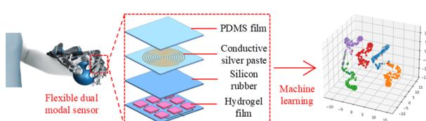
**Machine learning-assisted flexible dual modal sensor for multi-sensing detection and target object recognition in the grasping process**
