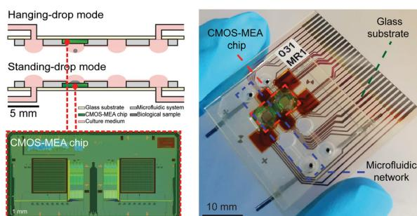
**Seamless integration of CMOS microsensors into open microfluidic systems**
