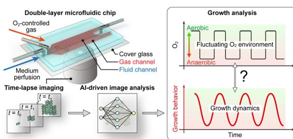
**Unveiling microbial single-cell growth dynamics under rapid periodic oxygen oscillations**
