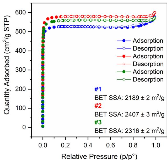
**Fig. 4**  $\text{N}_2$  adsorption–desorption isotherms at 77 K for the three batches of Ce-UiO-67-5% BPyDC: #1 in blue, #2 in red and #3 in green, respectively. For the sake of clarity, we have selected one of each three adsorption points up to  $150 \text{ cm}^3 \text{g}^{-1}$  STP and then one every other.
