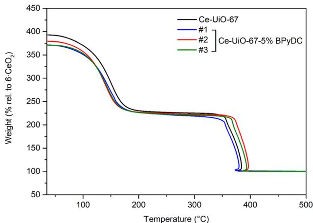
Fig. 3 TGA profiles of the three batches of Ce-UiO-67-5% BPyDC, #1 (blue line), #2 (red line) and #3 (green line), compared to that of Ce-UiO-67 (black line), reported as weight loss (%) related to  $\text{CeO}_2$ , set as 100%.
