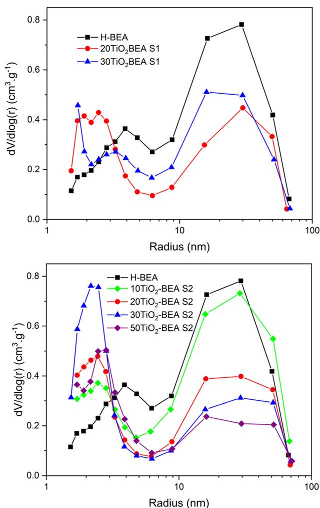
**Fig. 4** Pore size distribution curves (BJH, desorption branch) of TiO<sub>2</sub>-BEA composites: (top) S1 series and (bottom) S2 series.
