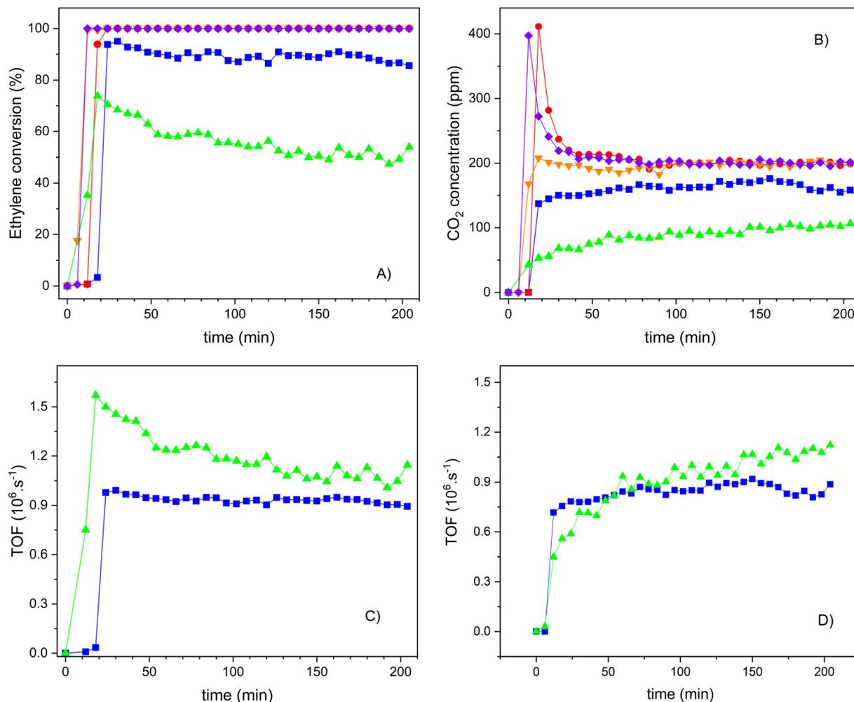
Fig. 13 Ethylene photooxidation experiments under UVA-vis irradiation for S2 series samples: A) ethylene conversion; B) CO<sub>2</sub> concentration; C) TOF values (calculated from ethylene); and D) TOF values (calculated from CO<sub>2</sub>) (10TiO<sub>2</sub>-BEA S2 (▲), 20TiO<sub>2</sub>-BEA S2 (■), 30TiO<sub>2</sub>-BEA S2 (●), 50TiO<sub>2</sub>-BEA S2 (◆) and TiO<sub>2</sub>-S2 (▼); experimental conditions: C<sub>2</sub>H<sub>4</sub> 100 ppm, 25 cm<sup>3</sup> min<sup>-1</sup>, 0.45 g).
