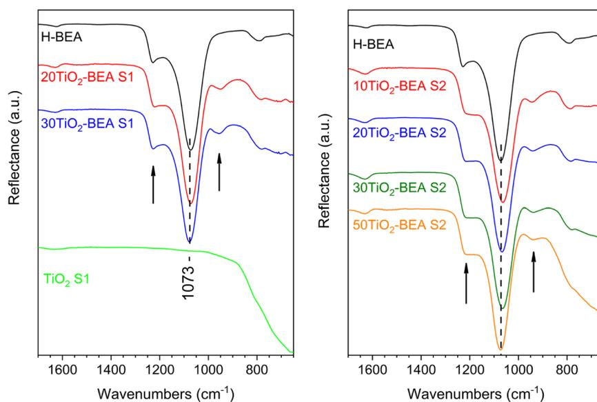
Fig. 6 FTIR spectra of the different composite materials (ATR mode): (left), S1 series, and (right) S2 series (the arrows in both figures depict the bands at about 1230 and 950 cm<sup>-1</sup>).
