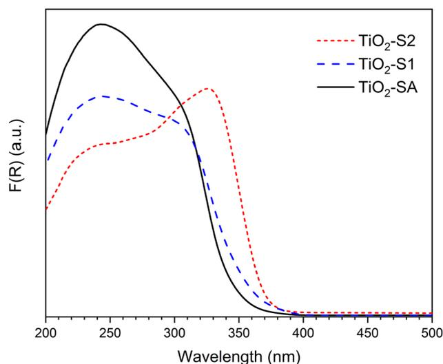
**Fig. 2** UV-vis DRS spectra of bulk TiO<sub>2</sub> samples: TiO<sub>2</sub>-SA (black), TiO<sub>2</sub>-S1 (blue) and TiO<sub>2</sub>-S2 (red).
