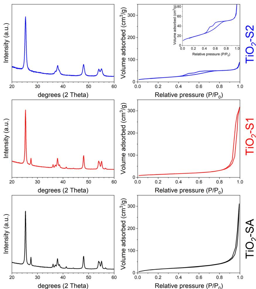
**Fig. 1** (Left) PXRD patterns and (right) N<sub>2</sub> isotherms (at 77 K) of bulk TiO<sub>2</sub> samples: TiO<sub>2</sub>-SA (black), TiO<sub>2</sub>-S1 (red) and TiO<sub>2</sub>-S2 (blue). Inset: details of the TiO<sub>2</sub>-S2 isotherm.
