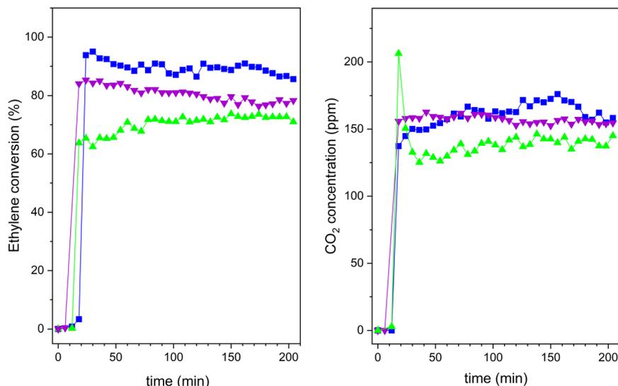
**Fig. 12** Ethylene photooxidation experiments under UVA-vis irradiation for 20TiO<sub>2</sub>-BEA S2 (■); 20TiO<sub>2</sub>-BEA S1 (▲) and 30TiO<sub>2</sub>-BEA S1 (▼): (left) ethylene conversion; (right) CO<sub>2</sub> concentration (experimental conditions C<sub>2</sub>H<sub>4</sub> 100 ppm, 25 cm<sup>3</sup> min<sup>-1</sup>, 0.45 g).
