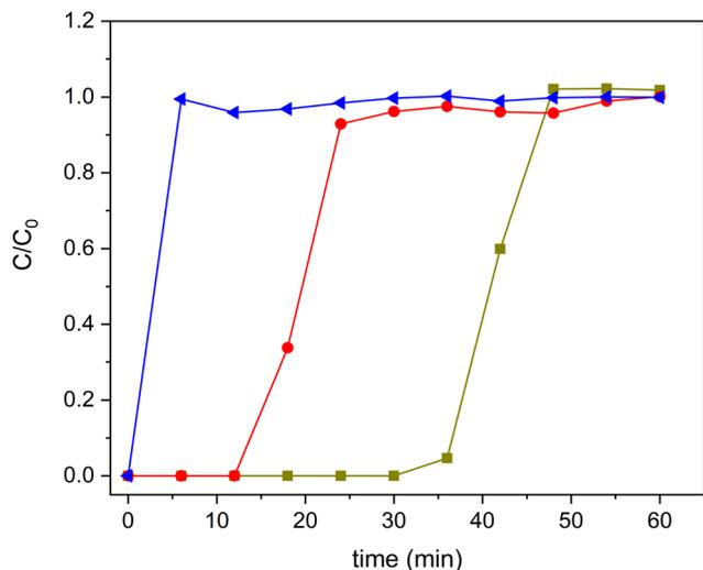
Fig. 10 Ethylene adsorption curves for samples H-BEA (■), 20TiO<sub>2</sub>-BEA S2 (●) and TiO<sub>2</sub>-S2 (◄) (C<sub>2</sub>H<sub>4</sub> 100 ppm, 25 cm<sup>3</sup> min<sup>-1</sup>, RT).
