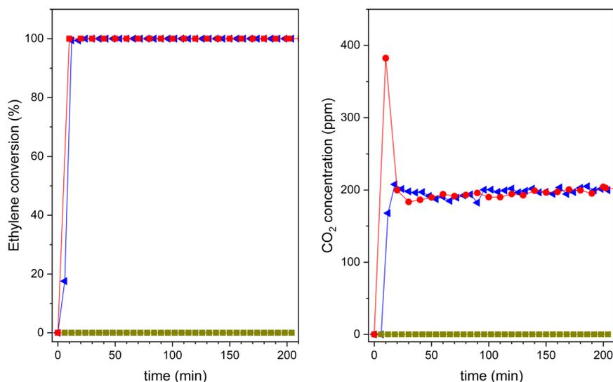
Fig. 11 Ethylene photooxidation experiments under UV-vis light for H-BEA (■), 20TiO<sub>2</sub>-BEA S2 (●) and TiO<sub>2</sub>-S2 (◄): (left) ethylene conversion; (right) CO<sub>2</sub> concentration (experimental conditions C<sub>2</sub>H<sub>4</sub> 100 ppm, 25 cm<sup>3</sup> min<sup>-1</sup>, 0.45 g).
