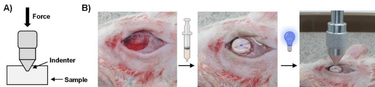
Fig. 4 (A) Schematic overview of the indentation test, (B) ex vivo indentation test of the fixated rat calvariae .
