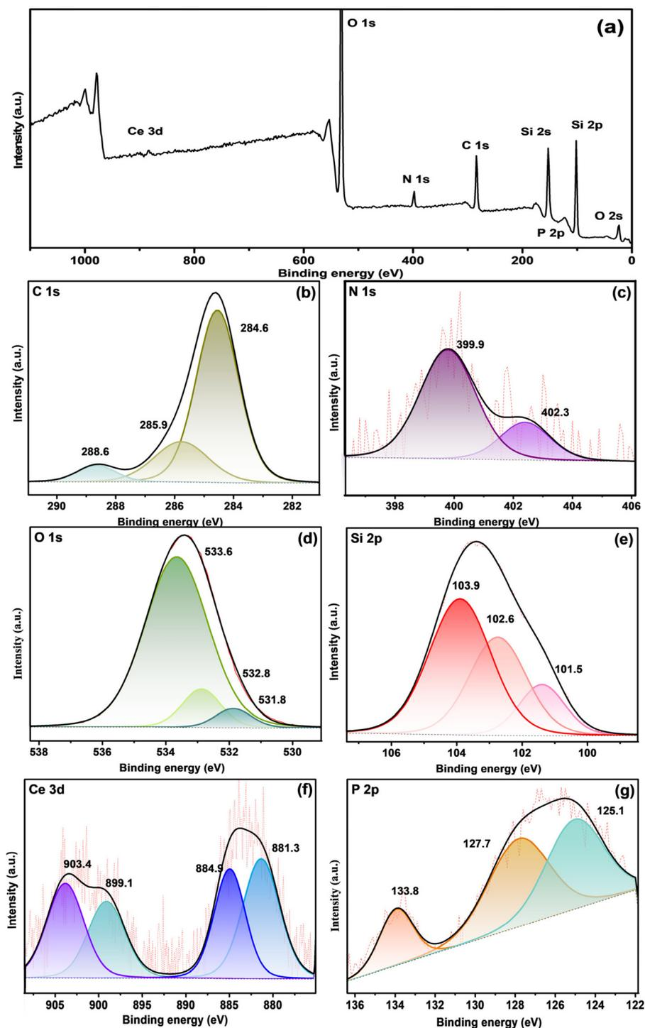
Fig. 6 (a) XPS survey spectrum fCP-SiO<sub>2</sub> and High-resolution XPS spectra of (b) C 1s, (c) N 1s, (d) O 1s, (e) Si 2p, (f) Ce 3d and (g) P 2p orbitals.
