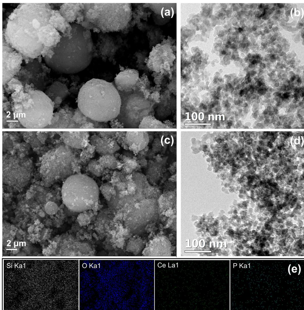
Fig. 4 Micrograph of silica and CP-SiO<sub>2</sub> (a and c), SEM images (b and d), TEM images and (e) SEM elemental mapping of CP-SiO<sub>2</sub>.
