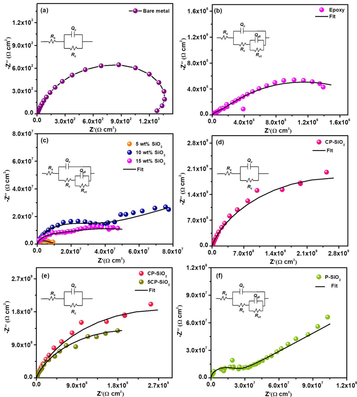
**Fig. 7** Nyquist plots of (a) bare steel coupon, (b) bare epoxy coating, (c) silica loaded (5, 10 and 15 wt%) epoxy coatings, (d) 10 wt% of hybrid pigment CP-SiO<sub>2</sub> epoxy coating, (e) different compositions of CP-SiO<sub>2</sub> (10 wt%) loaded epoxy coatings and (f) 10 wt% of P-SiO<sub>2</sub> epoxy coating (electrochemical equivalent circuit given in the inset of Nyquist plots).
