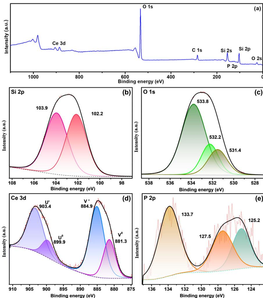
Fig. 3 XPS spectra of CP-SiO<sub>2</sub> (a) and survey and high-resolution spectra of (b) Si 2p, (c) O 1s, (d) Ce 3d and (e) P 2p.
