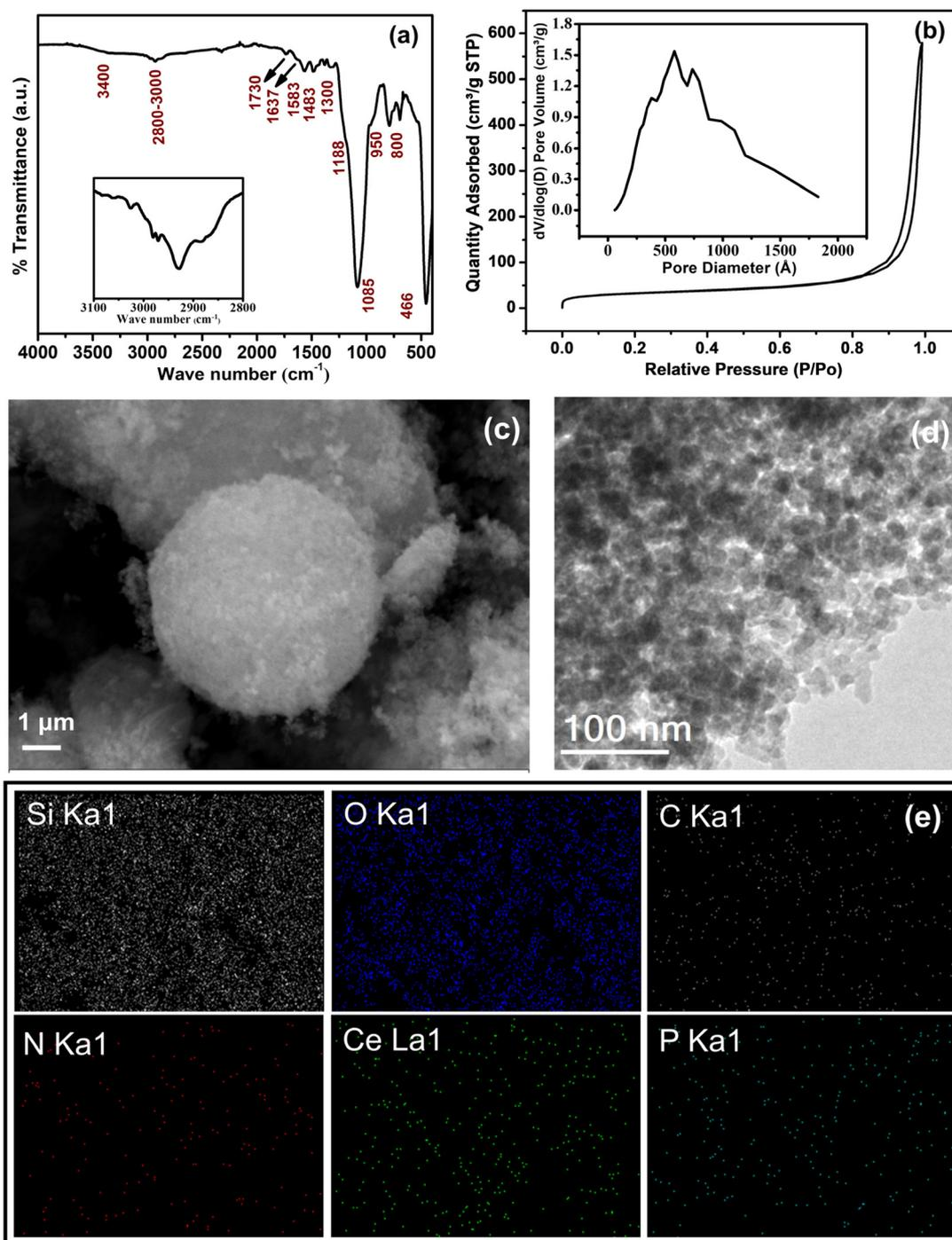
**Fig. 5** (a) IR spectra, (b)  $N_2$  adsorption and desorption isotherms from BET analysis with the inset showing BJH pore size distribution, (c) SEM image, (d) TEM image and (e) SEM elemental mapping of fCP-SiO<sub>2</sub>.
