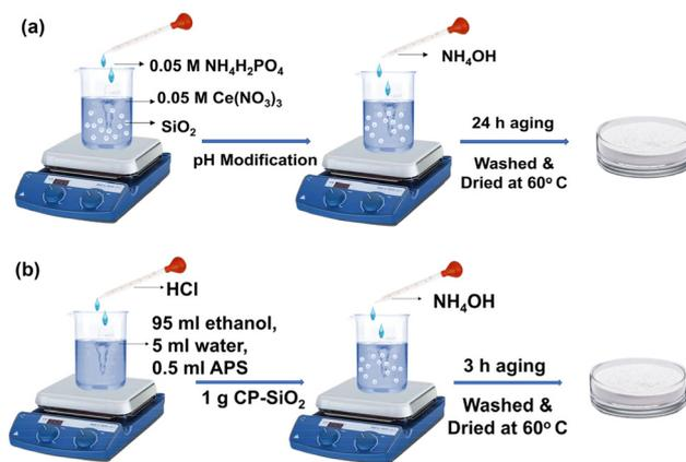
Fig. 1 Schematic illustration of (a) CP-SiO<sub>2</sub> preparation and (b) functionalisation of CP-SiO<sub>2</sub>.
