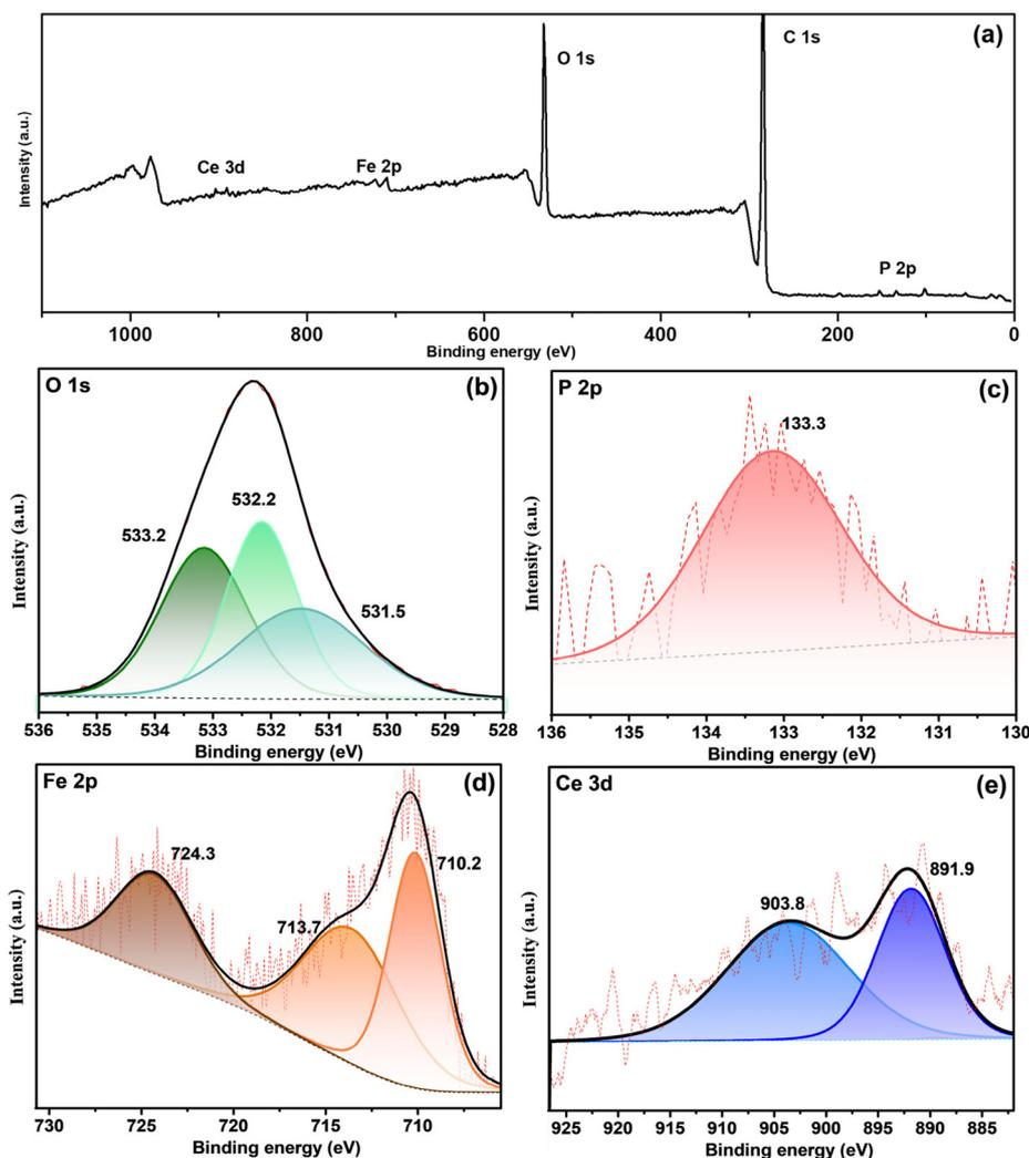
Fig. 9 XPS curve fitting of (a) the survey spectrum. (b) O 1s, (c) P 2p, (d) Fe 2p and (e) Ce 3d of the inhibitive film beneath the CP-SiO<sub>2</sub> loaded epoxy coating on steel depart from the 3.5 wt% NaCl solution.
