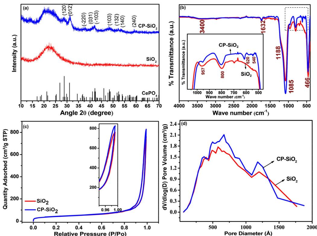
Fig. 2 (a) PXRD pattern, (b) IR spectra, (c)  $\text{N}_2$  adsorption and desorption isotherms from BET analysis and (d) BJH pore size distribution of silica and hybrid pigment CP-SiO<sub>2</sub>.
