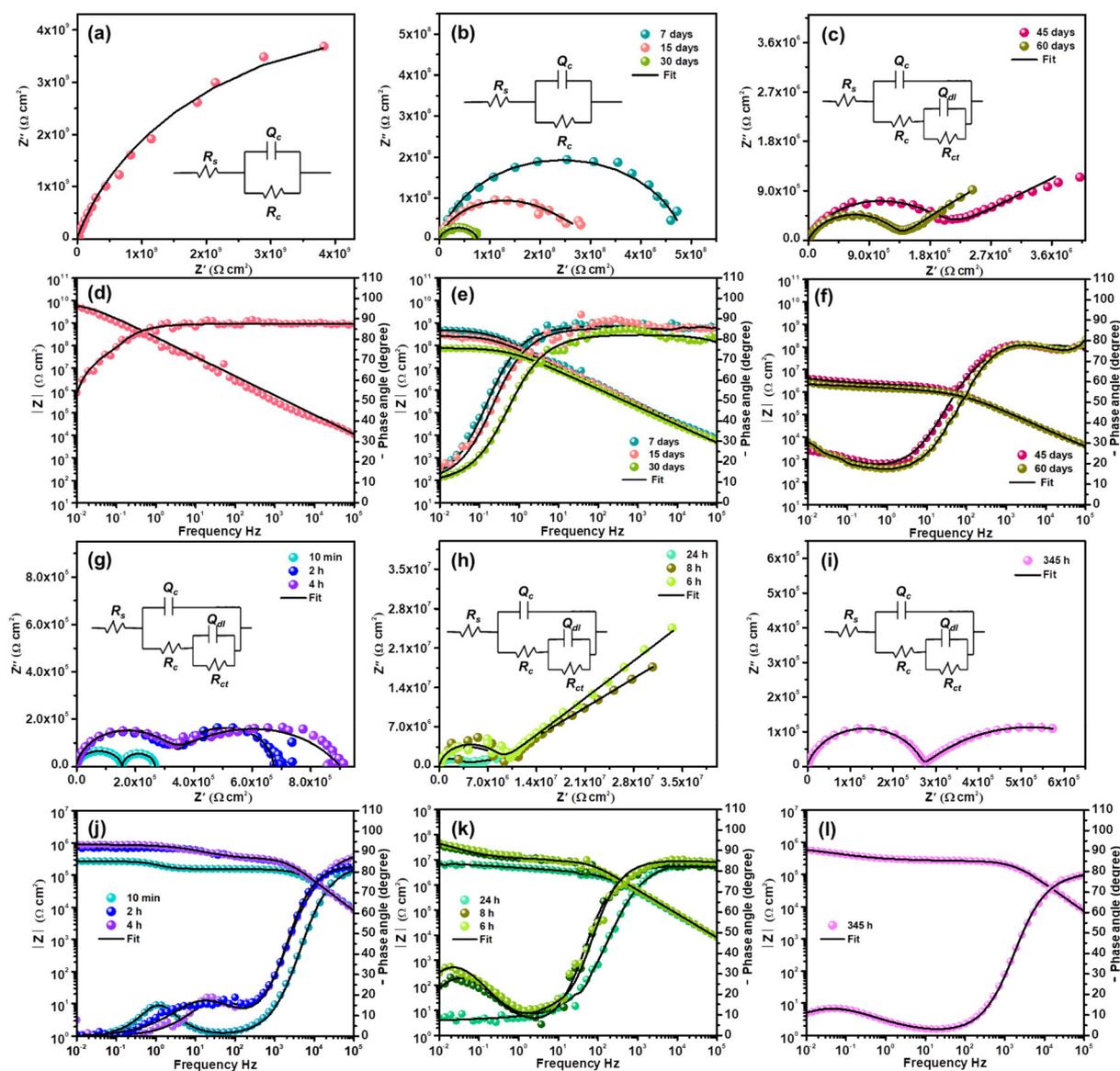
**Fig. 8** Continuous EIS study of the fCP-SiO<sub>2</sub> loaded epoxy-polyamide coating in 3.5% NaCl solution (a–f) and without artificial defect and (g–l) artificial defect coating (electrochemical equivalent circuit given in the inset of Nyquist plots).
