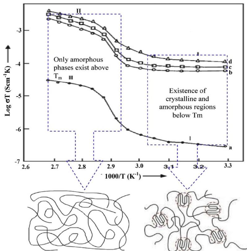
**Fig. 19** Temperature dependence of dc conductivity of (a) pure PEO, (b) (PEO + NaClO<sub>3</sub>) (90 : 10), (c) (PEO + NaClO<sub>3</sub>) (80 : 20), and (d) (PEO + NaClO<sub>3</sub>) (70 : 30). Reprinted with permission from ref. 141. Copyright Elsevier 2006 (license number: 5677791086137).
