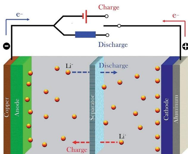
Fig. 1 Schematic mechanism of Li<sup>+</sup> ion battery. Reprinted with permission from ref. 7. Copyright Elsevier 2008 (license number: 5673181018376).
