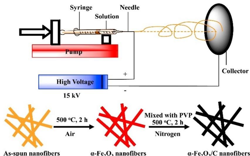
**Fig. 10** Schematic illustration of producing polymer-based nanofibers through the electrospinning process. Reprinted with permission from ref. 103. Copyright Elsevier 2016 (license number: 5673190990510).
