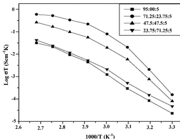
Fig. 18 Temperature dependence of ionic conductivity for PVAc:PVdF:LiClO<sub>4</sub> polymer electrolytes containing various blend ratios. Reprinted with permission from ref. 140. Copyright Elsevier 2006 (license number: 5677261076435).
