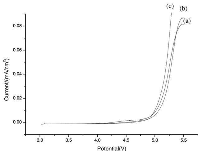
**Fig. 24** LSV of the PEO-based CPE at 60 °C. Salt content is  $[\text{LiClO}_4]/[\text{EO}] = 0.1$  and inorganic filler is 10 wt%. (a)  $\text{Al}_2\text{O}_3$  activated acid; (b)  $\text{Al}_2\text{O}_3$  activated neutral; (c)  $\text{Al}_2\text{O}_3$  activated basic. Reprinted with permission from ref. 113. Copyright Elsevier 2003 (license number: 5677800798772).
