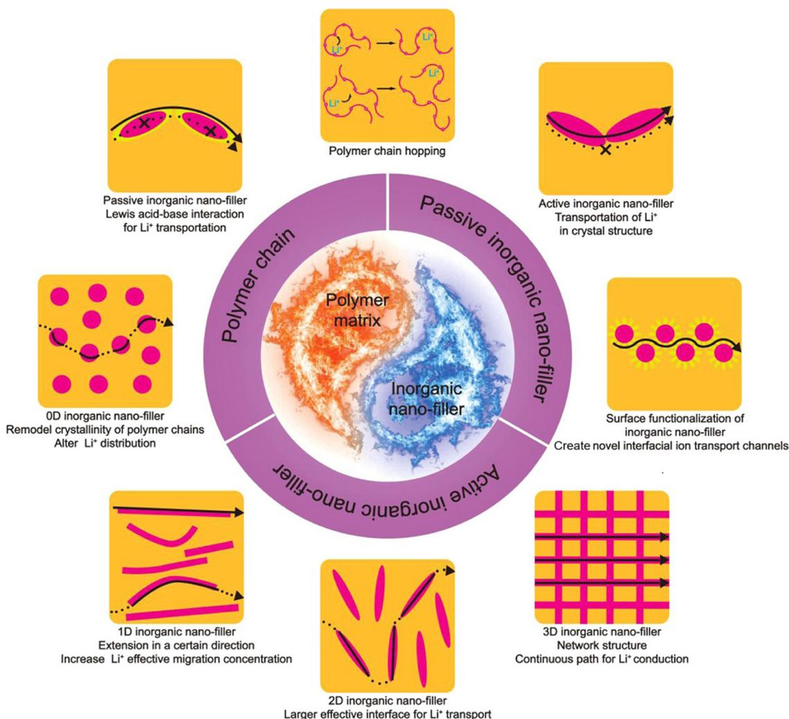
**Fig. 6** Schematic representation of various types of inorganic fillers and their function in ion transport. Reused with permission from ref. 82. Copyright Carbon Energy 2021 (open access CC-BY license 4.0).
