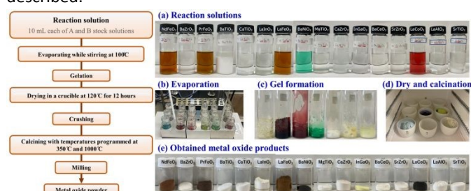
Figure 1: Schematic illustration of the catalyst synthesis process with pictorial representation.
