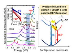
Near-bandgap emission in [HOC<sub>2</sub>H<sub>4</sub>NH<sub>3</sub>]<sub>2</sub>Pbl<sub>4</sub> perovskite under hydrostatic pressure: emission of a free exciton and a polaronic exciton
