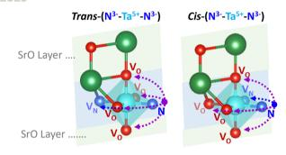
Influence of anion ordering on defect diffusion anisotropy in layered perovskite Sr<sub>2</sub>TaO<sub>3</sub>N: implications for oxynitride stability
