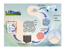
N/O co-doped porous carbon derived from polyester waste for electrochemical production of H<sub>2</sub>O<sub>2</sub>
