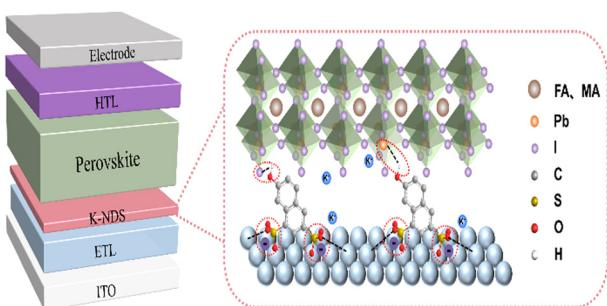
**Synergistic dual-layer passivation boosts efficiency and stability in perovskite solar cells using naphthal sulfonate**
