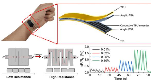
**Highly sensitive strain sensors with ultra-low detection limit based on pre-defined serpentine cracks**
