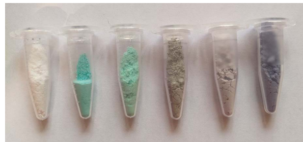
Fig. 10 Pictures of LDHs powders, from left to right: Mg/Al, MgNi/Al, MgNi/AlIn, MgNiCo/AlIn, MgNiCo/AlInSc, and MgNiCo/AlInScTm.
