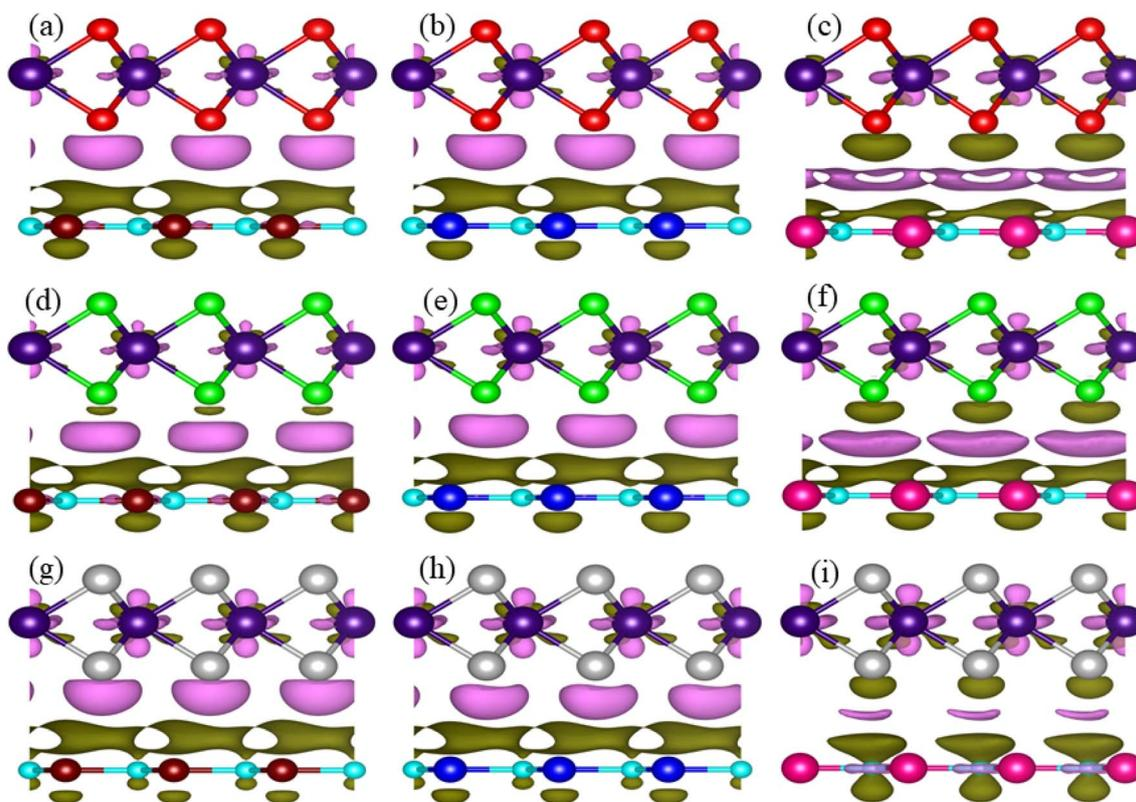
Fig. 9 Charge density difference of (a) TaS<sub>2</sub>-BP, (b) TaS<sub>2</sub>-BAS, (c) TaS<sub>2</sub>-BSb, (d) TaSe<sub>2</sub>-BP, (e) TaSe<sub>2</sub>-BAS, (f) TaSe<sub>2</sub>-BSb, (g) TaTe<sub>2</sub>-BP, (h) TaTe<sub>2</sub>-BAS, and (i) TaTe<sub>2</sub>-BSb, MS vdWHs.
