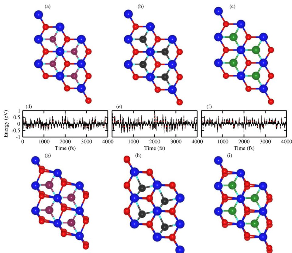
**Fig. 3** *Ab initio* molecular dynamics simulation of (a, d, and g)  $\text{TaS}_2\text{-BP}$ , (b, e, and h)  $\text{TaS}_2\text{-BAS}$  and (c, f, and i)  $\text{TaS}_2\text{-BSb}$ , van der Waals heterostructures. Geometrical structure (a–c) before heating; (g–i) after heating with (d–f) fluctuating energy.
