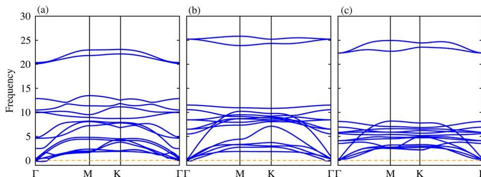
Fig. 4 Phonon dispersion curves of (a) TaS<sub>2</sub>-BP, (b) TaS<sub>2</sub>-BAs and (c) TaS<sub>2</sub>-BSb MS vdWHs.
