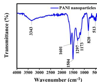
Fig. 4 FT-IR spectra of pure PANI nanoparticles.
