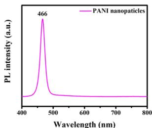
Fig. 5 Photoluminescence (PL) of standard pristine polyaniline nanoparticles.
