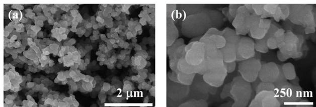
Fig. 1 (a) Low-, (b) high-magnification SEM of the annealed pure polyaniline (PANI).
