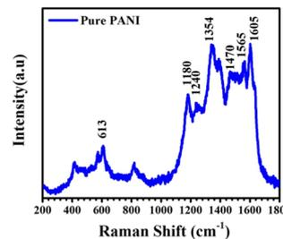
Fig. 3 Raman spectrum of pure PANI nanoparticles.
