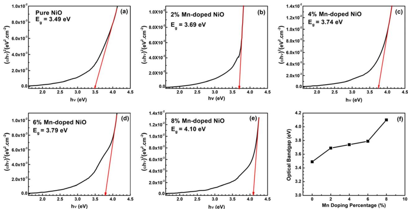
Fig. 6 Tauc plot of the Ni<sub>1-x</sub>Mn<sub>x</sub>O NPs: (a)  $x = 0$ , (b)  $x = 0.02$ , (c)  $x = 0.04$ , (d)  $x = 0.06$ , (e)  $x = 0.08$ . And variation of NiO NPs optical bandgap with different Mn doping concentrations (f).
