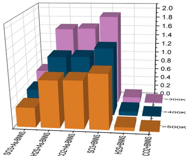
Fig. 4 Sensitivity of gas adsorbed BNNS and As-BNNS structures at different temperatures.
