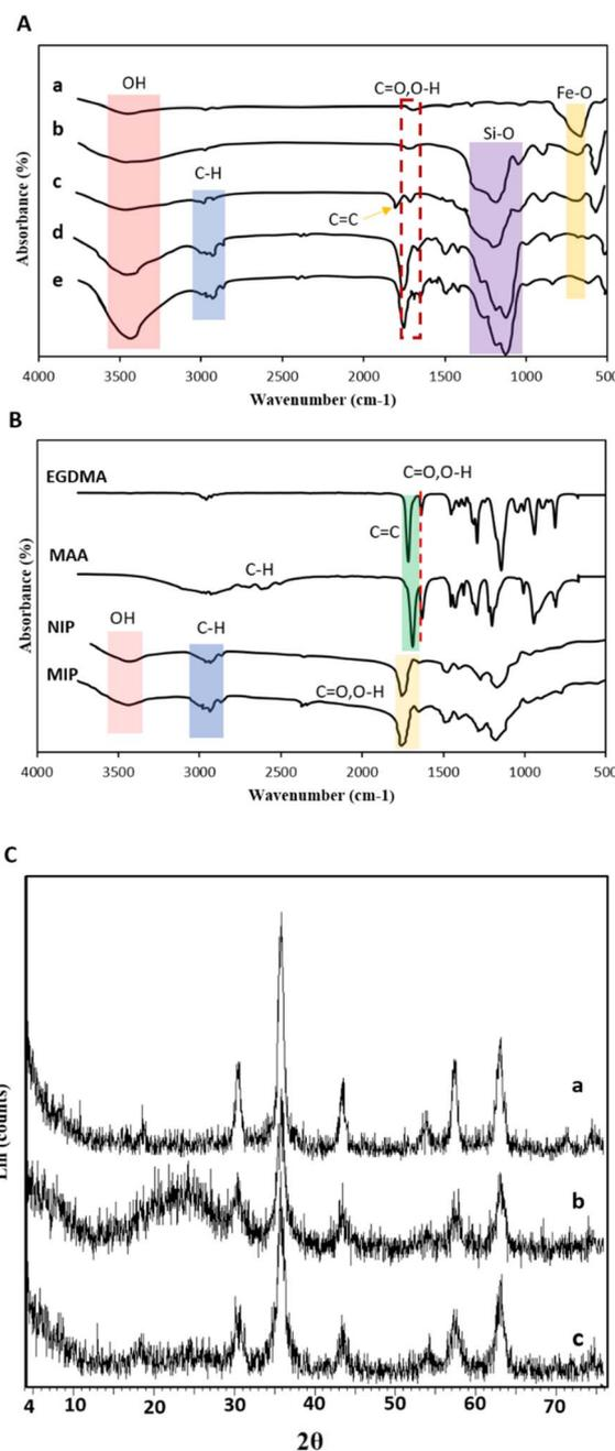
Fig. 1 (A) FTIR spectra of (a) Fe<sub>3</sub>O<sub>4</sub>, (b) Fe<sub>3</sub>O<sub>4</sub>@SiO<sub>2</sub>, (c) Fe<sub>3</sub>O<sub>4</sub>@SiO<sub>2</sub>@TMSPMA, (d) MNIPs and (e) MMIPs; (B) FTIR spectra of the monomer, crosslinker, MIPs and NIPs; (C) XRD patterns of (a) Fe<sub>3</sub>O<sub>4</sub>, (b) Fe<sub>3</sub>O<sub>4</sub>@SiO<sub>2</sub>, and (c) Fe<sub>3</sub>O<sub>4</sub>@SiO<sub>2</sub>@TMSPMA.
