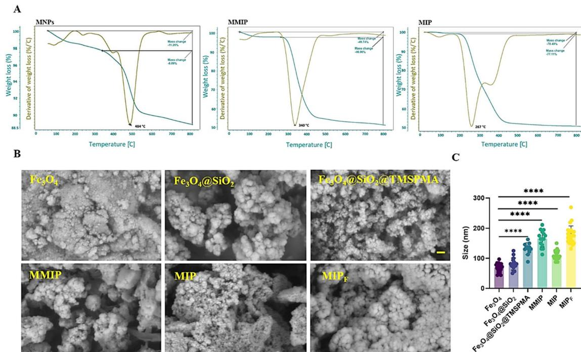
Fig. 2 (A) TGA thermograms of MNPs, MMIPs, MIPs. (B) SEM images; the scale bar is 300 nm. (C) Size of nanocomposites. Data were used as mean  $\pm$  SD, and  $P$  values were \*\*\*\* $p < 0.0001$  for all carriers by one-way ANOVA.
