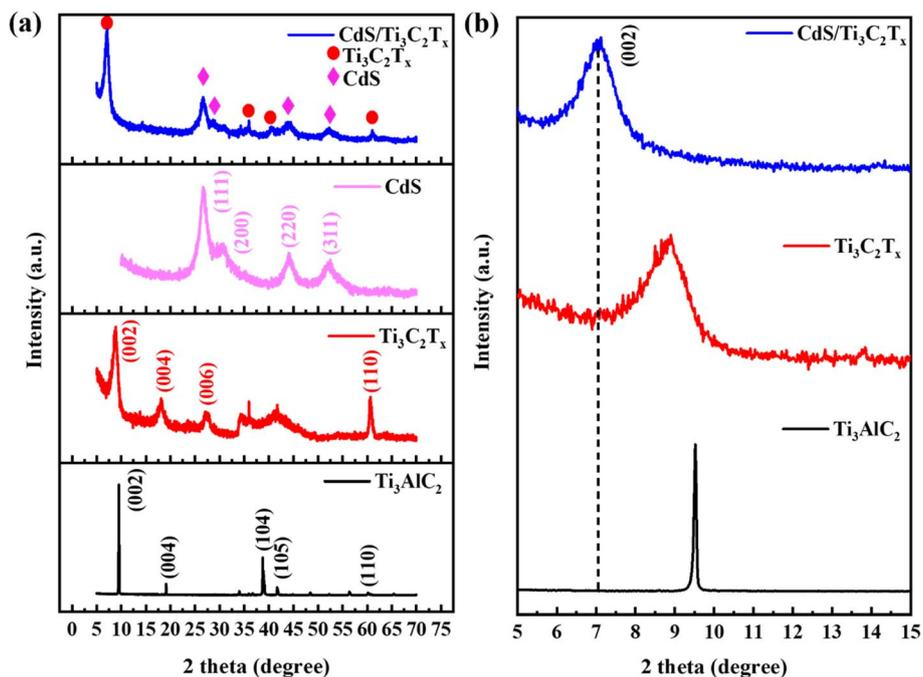
Fig. 4 (a) High angle and (b) low angle XRD patterns of  $\text{Ti}_3\text{AlC}_2$  powder,  $\text{Ti}_3\text{C}_2\text{T}_x$  MXene, mesoporous CdS nanoparticle, and the CdS/ $\text{Ti}_3\text{C}_2\text{T}_x$  heterostructure.
