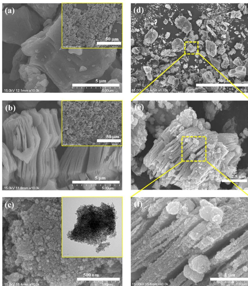
Fig. 2 SEM images of (a) pristine  $\text{Ti}_3\text{AlC}_2$ , (b)  $\text{Ti}_3\text{C}_2\text{T}_x$  MXene, (c) CdS (the inset figure is the TEM of CdS) and (d–f) the CdS/ $\text{Ti}_3\text{C}_2\text{T}_x$  heterostructure.
