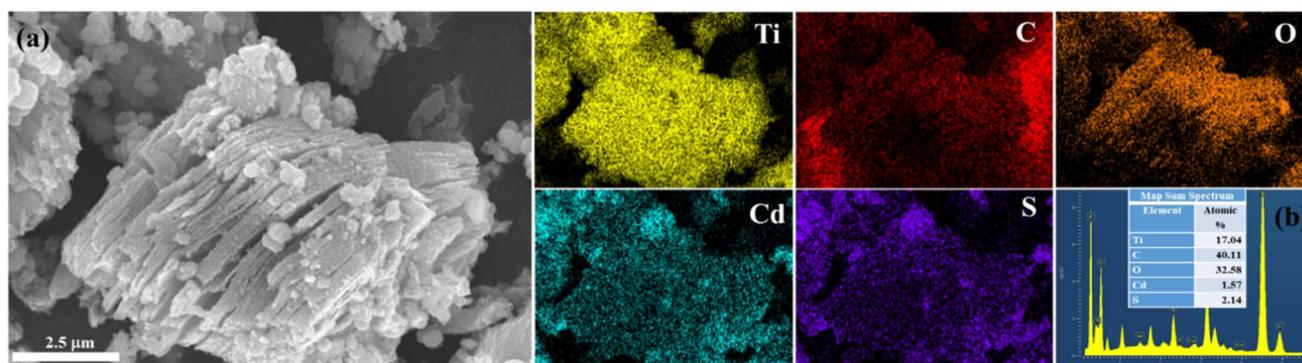
Fig. 3 (a) SEM images and (b) SEM-EDX elemental mapping of the CdS/ $\text{Ti}_3\text{C}_2\text{T}_x$  heterostructure.
