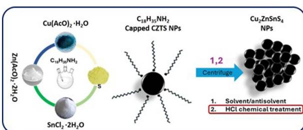
**Optimized hot injection and HCl purification for high quality Cu<sub>2</sub>ZnSnS<sub>4</sub> nanoparticles**
