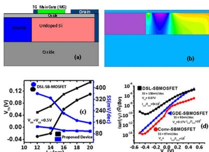
**Optimized nano-scaled drain- and gate-engineered Schottky barrier MOSFET with improved ambipolarity and RF characteristics**
