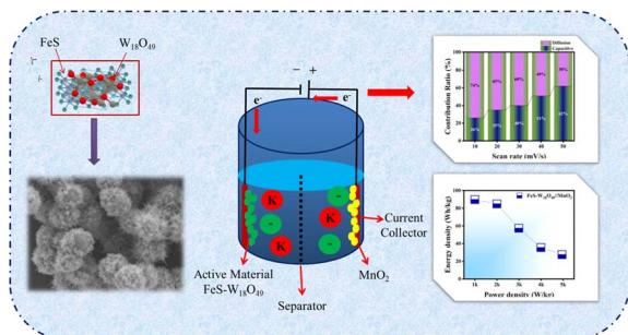
**First investigation of high-performance FeS-based W<sub>18</sub>O<sub>49</sub> asymmetric supercapacitors operating at 1.6 V**
