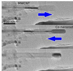
**Electromigration-driven linear actuator operations of Co nanorods inside and outside multi-walled carbon nanotubes with stroke of tens of nanometers**
