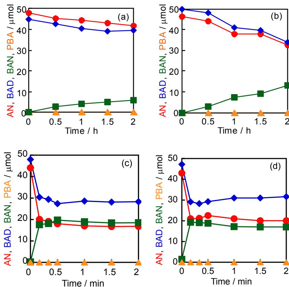
**Fig. 2** Production of BAN (■) by condensation of AN (●) and BAD (◆) in 2-propanol suspensions under various conditions: (a) with no additive, (b) in the presence of 1wt% Au-C<sub>3</sub>N<sub>4</sub> (50 mg), (c) in the presence of OA (100  $\mu\text{mol}$ ), and (d) in the presence of OA (100  $\mu\text{mol}$ ) and 1wt% Au-C<sub>3</sub>N<sub>4</sub> (50 mg). PBA (▲) was not produced in all cases.
