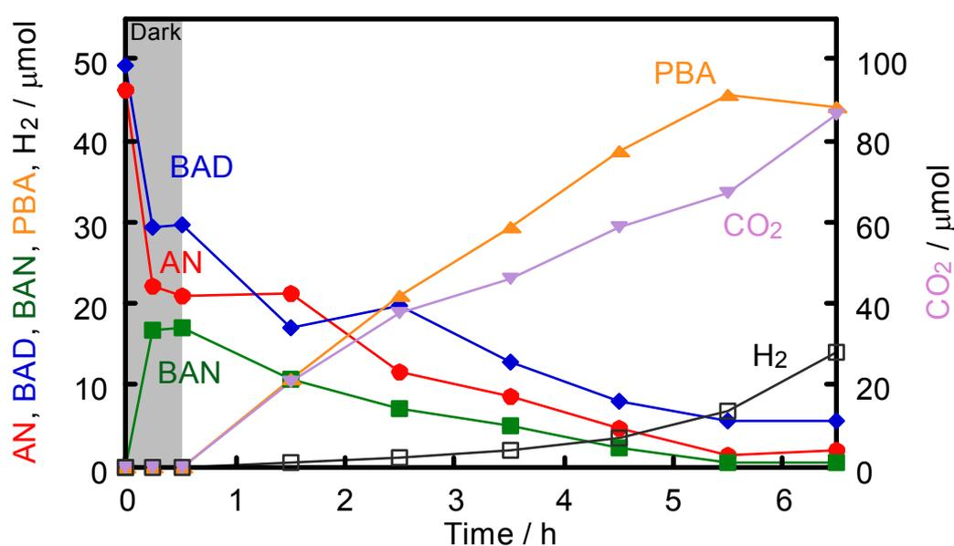
**Fig. 3** Time courses of the amounts of BAD (◆), AN (●), BAN (■), PBA (▲), CO<sub>2</sub> (▼) and H<sub>2</sub> (□) in a 2-propanol suspension of Au-C<sub>3</sub>N<sub>4</sub> in the presence of OA as an
