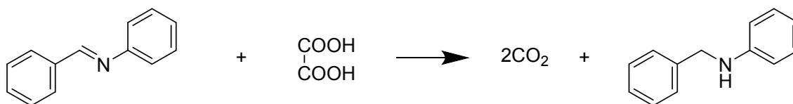
**Scheme 2** Photocatalytic reaction of BAN and OA to PBA and CO<sub>2</sub>.
