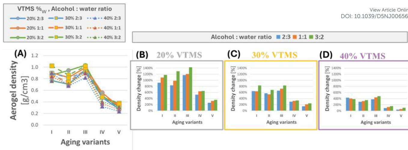
**Figure 7.** (A) Apparent density of the obtained aerogels, depending on the synthesis composition and the aging variant, (B-D) change in density of aerogel compared to the gel after gelation, for different precursor concentrations: 20%, 30%, and 40% respectively
