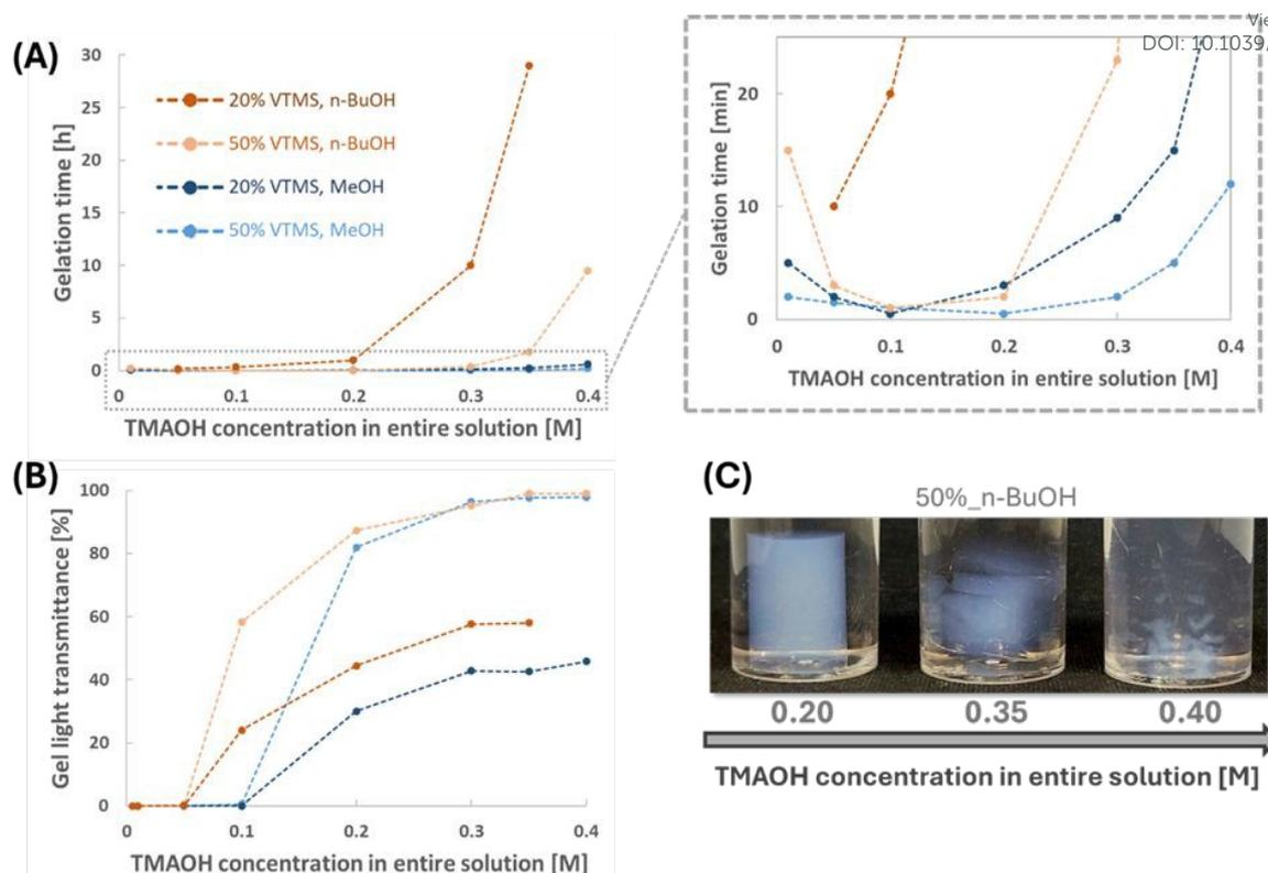
**Figure 2.** (A) Gelation time for different TMAOH and VTMS concentrations and solvent types (with a detailed view of a particular period), (B) VTMS-based gels light transmittance for different TMAOH and VTMS concentration and solvent type, (C) Dissolution phenomenon depending on the TMAOH concentration
