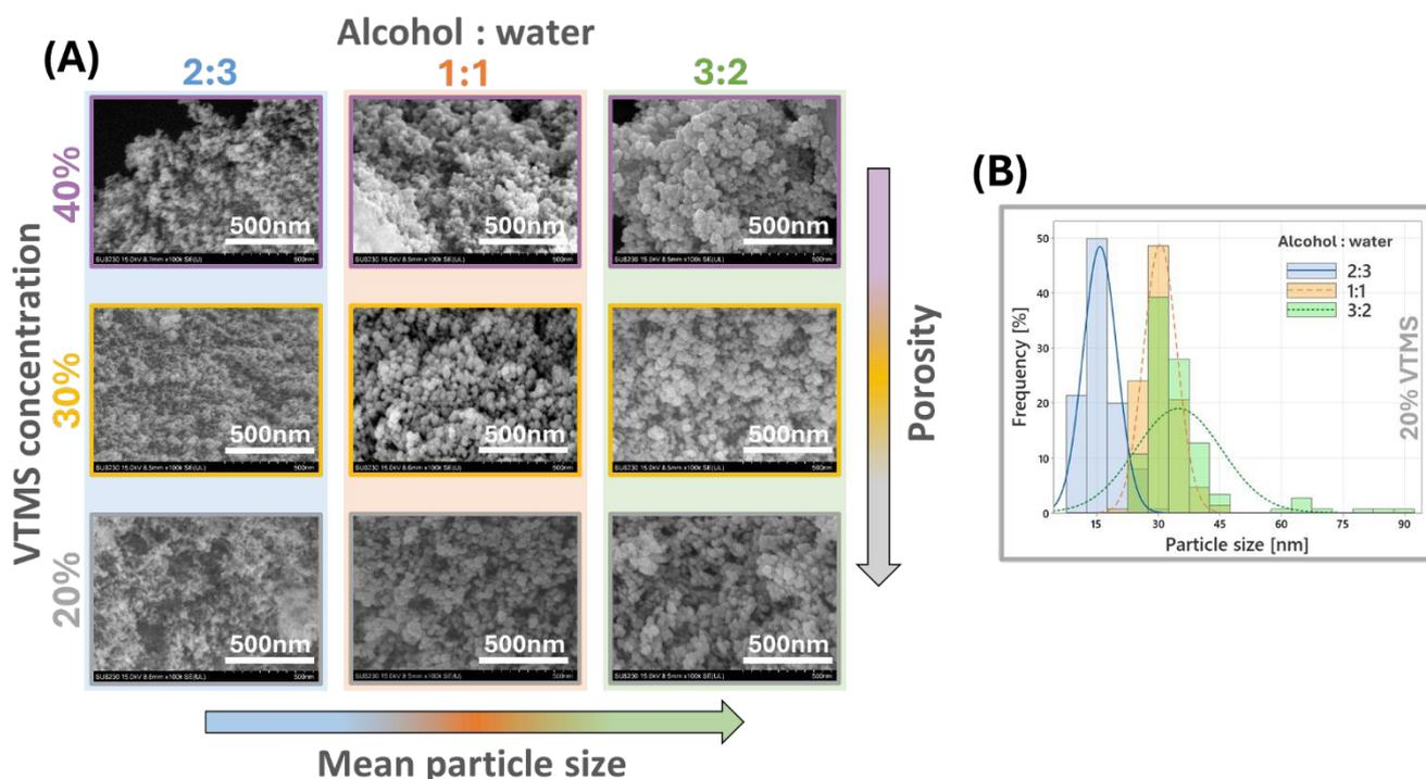
**Figure 3.** (A) SEM images - approximated x100k - of aerogels obtained from different synthesis compositions, (B) histogram of particle size distribution for samples with 20%<sub>w</sub> VTMS and different alcohol-to-water ratios in the synthesis
