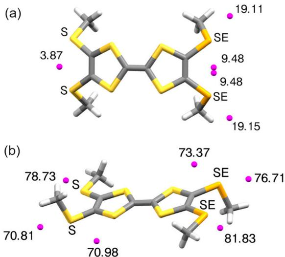
Fig. 6 Localization (pink dots) and maximum values of  $V_{s,max}$  in the vicinity of the outer S and Se atoms in (a) **1** and (b) **1**<sup>•+</sup> determined on geometry-optimized molecules (DFT, B3LYP/def2TZVP/D3).
