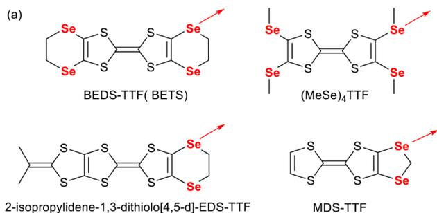
**Scheme 1** Reported selenated TTFs engaged in ChB interactions in their salts. The red arrow shows the direction of the expected ChB interaction toward Lewis bases upon the activation of TTF through oxidation.
