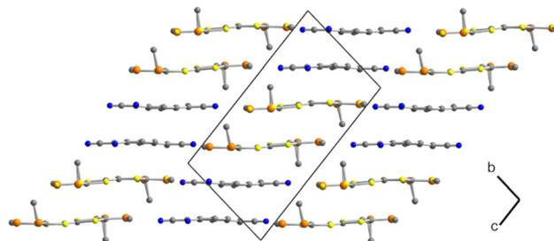
Fig. 2 Projection view along  $a$  of the unit cell of (**1**)-TCNQ showing the DDAADDAA stacking motif.
