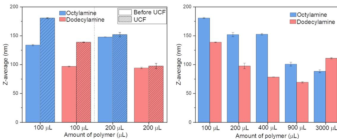
**Fig. 2** Hydrodynamic sizes of the polymer-coated NPs (*via* magnetic stirring) measured by DLS, before and after the ultracentrifugation step (left) and of all the samples after ultracentrifugation (right). The error bars represent the standard deviation determined from triplicate DLS measurements.
