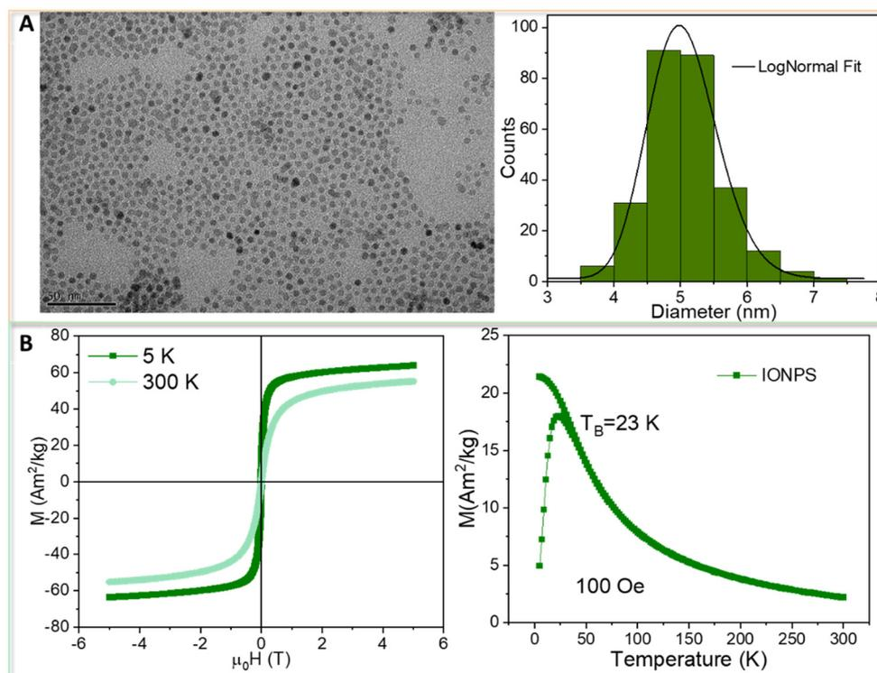
**Fig. 1** (A) TEM of the as-synthesized iron oxide nanoparticles and the size distribution fitted to a log-normal and (B) MH curves at 5 K and 300 K and ZFC-FC curves measured applying a magnetic field of 100 Oe.
