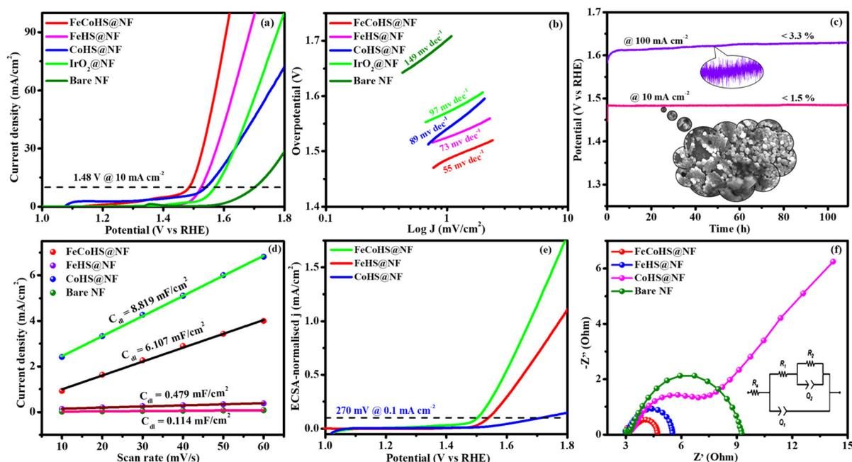
**Fig. 5** OER polarization curves of electrocatalysts: (a) LSV (without  $iR$ -correction); (b) Tafel plots; (c) chronopotentiometry durability test (inset: post OER image); (d) double-layer capacitance; (e) ECSA-normalized LSV curve and (f) Nyquist plot.
