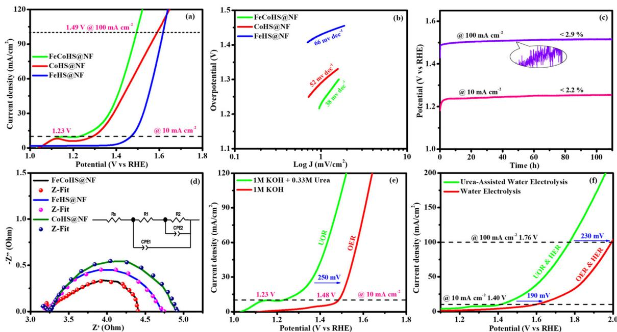
**Fig. 8** UOR polarization curves (without  $iR$  correction) of electrocatalysts: (a) LSV curve; (b) Tafel slopes; (c) chronopotentiometry durability test (inset: post HER image); (d) Nyquist plots (inset: Randles equivalent circuit); and (e and f) comparison of the LSV curve for the OER and electrolyzer with KOH.
