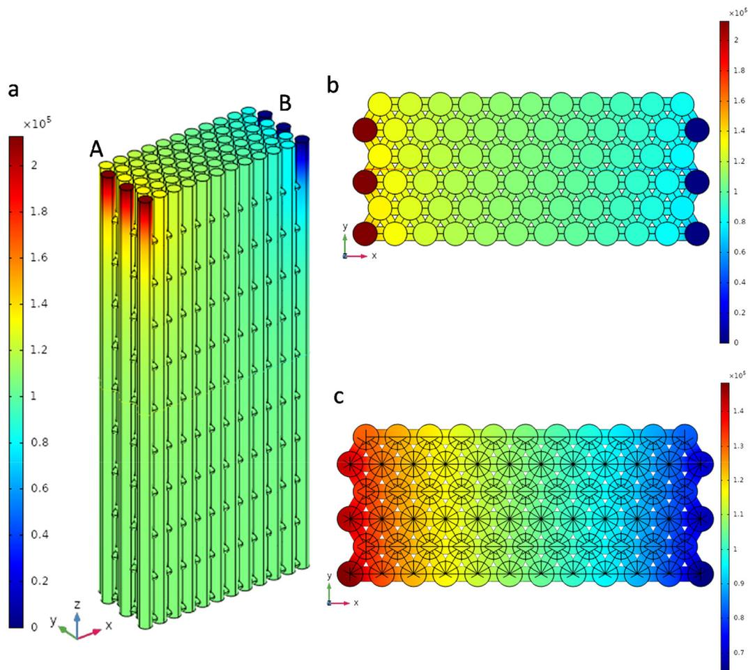
**Fig. 3** (a) Lateral perspective of the COMSOL geometry used in this simplified model of the measurement, once the simulation of the electrical conduction has been carried out, where the two terminals can be seen (A being the input terminal and B the ground), (b) top view of the COMSOL simulation of the electrical conduction, and (c) sectional view of the first plane of transversal channels, where the main voltage drop along the structure takes place.
