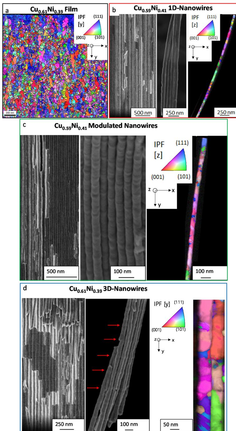
**Fig. 2** (a) PED orientation mapping of the CuNi film, SEM images inside AAO templates and after dissolving the AAO and transmission Kikuchi diffraction (TKD) images of (b) 1D-CuNi nanowires, (c) modulated-CuNi nanowires, and (d) 3D-CuNi nanonetworks both inside and outside the 3D-AAO template.
