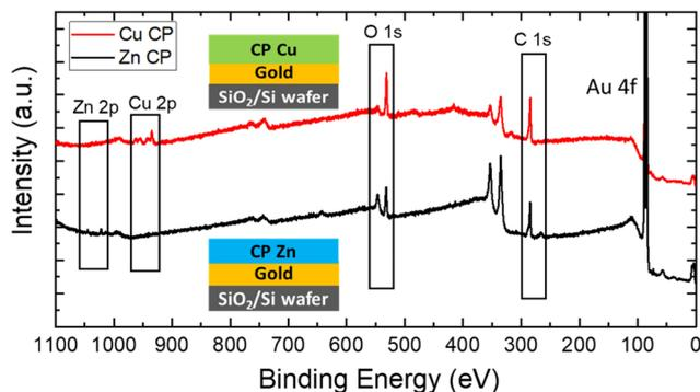
Fig. 3 XPS spectra of the Cu CP and Zn CP materials.
