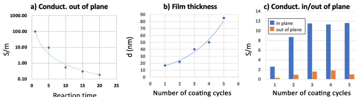
**Fig. 7** (a) Conductance of the Cu CP measured out-of-plane (*i.e.* vertically) vs. the reaction time (exposure to the ionic solution). (b) Increase of Cu CP film thickness with the number of OHPTP coating steps. (c) Conductance of the Cu CP measured in-plane (*i.e.*, horizontally) and out-of-plane (*i.e.*, vertically) with increasing film thickness. The dotted lines are just a guide for the eye.
