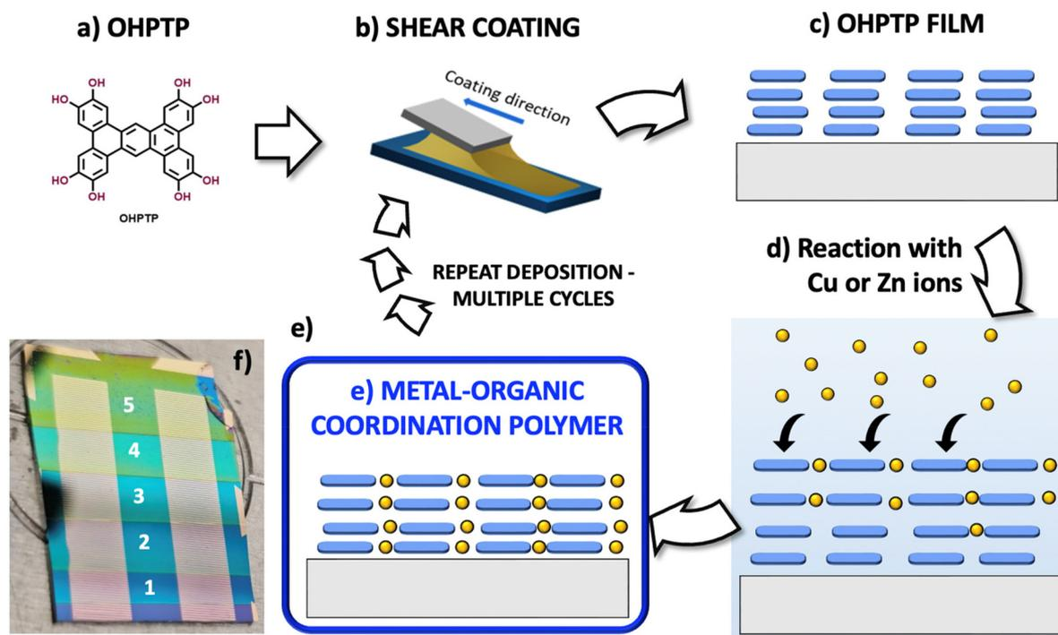
**Fig. 2** Scheme of the two-step procedure used to create the CP. (a) The organic building block OHPTP. (b) Shear coating of the organic molecules to obtain a uniform film (c), which is then dipped in a solution of Cu or Zn ions (d) to obtain the CP (e). (f) Photograph of a sample with uniform coatings obtained by multiple shear coating + dipping cycles; the white numbers indicate the number of cycles.
