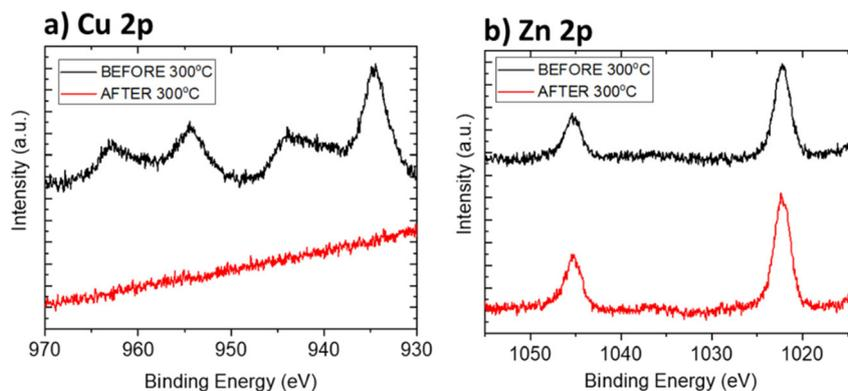
**Fig. 8** Thermal stability of the single-coated Cu and Zn thin films. XPS spectra recorded prior to any heating and after heating at  $300 \text{ }^\circ\text{C}$  in a vacuum for (a) the single-coated Cu thin film and (b) the single-coated Zn thin film.
