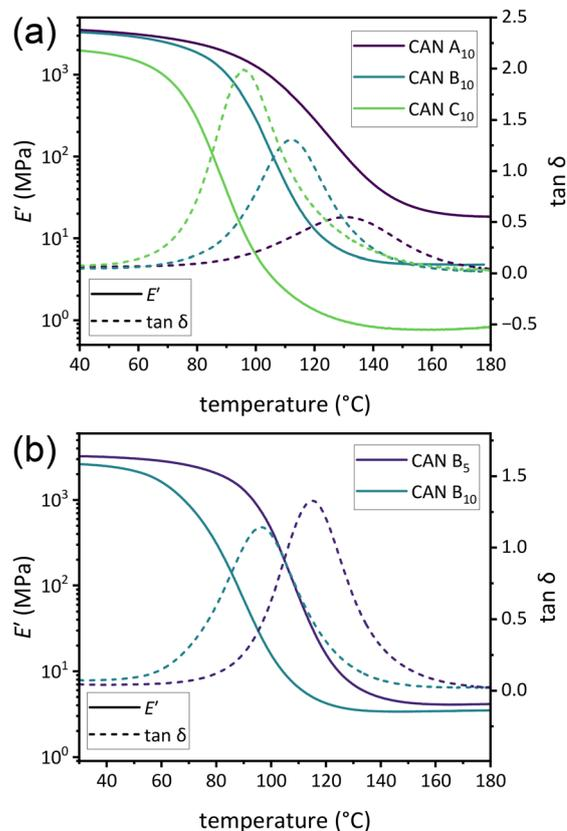
**Fig. 2** (a) DMA thermograms of  $E'$  versus temperature for CAN A<sub>10</sub>, CAN B<sub>10</sub>, and CAN C<sub>10</sub>. (b) DMA thermograms of  $E'$  and  $\tan \delta$  versus temperature for CAN B<sub>5</sub> and CAN B<sub>10</sub>.
