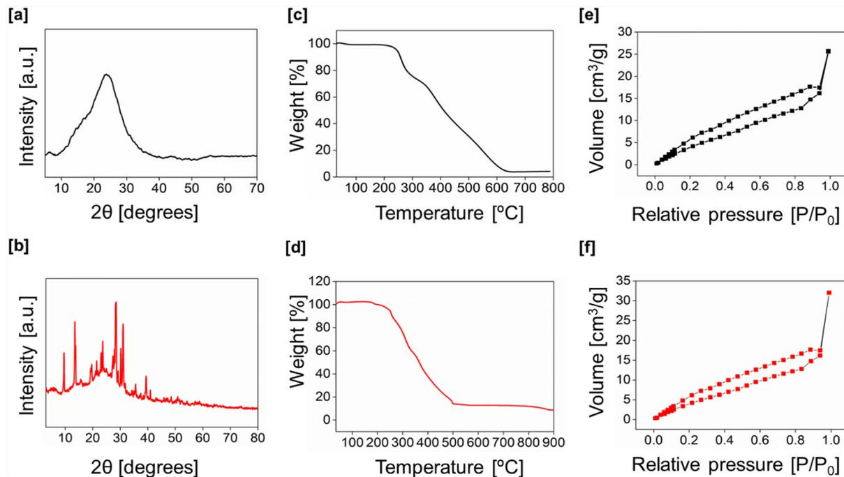
Fig. 2 pXRD pattern of [a] **gn-ipop-cl(ST)** and [b] **gn-ipop-cl(MC)**. TGA profile of [c] **gn-ipop-cl(ST)** and [d] **gn-ipop-cl(MC)**. BET surface area for [e] **gn-ipop-cl(ST)** and [f] **gn-ipop-cl(MC)**.
