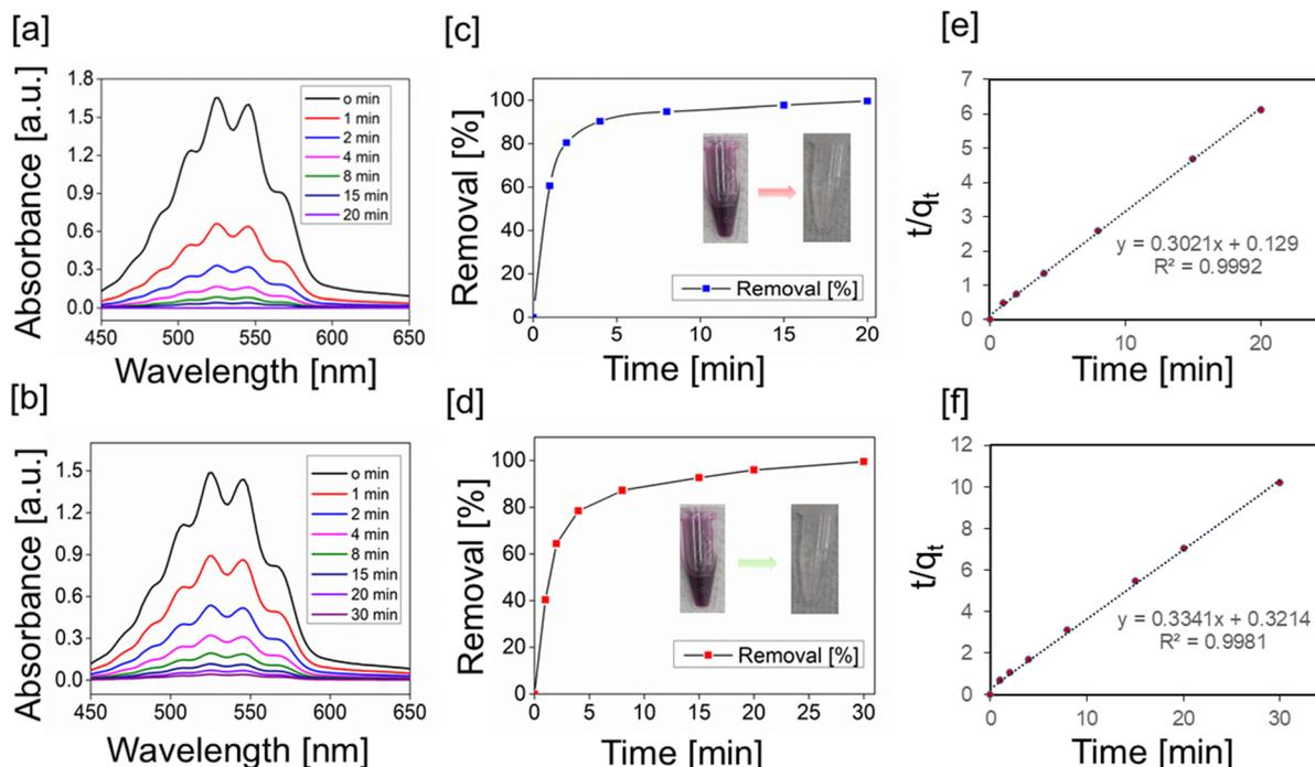
Fig. 4 UV-Vis spectra of  $\text{KMnO}_4$  demonstrating the rapid uptake of permanganate in the presence of [a] **gn-ipop-cl(MC)** and [b] **gn-ipop-cl(ST)**. Plot of time vs. % removal of [c] **gn-ipop-cl(MC)** and [d] **gn-ipop-cl(ST)**. Second-order fitting for  $\text{KMnO}_4$  adsorption for [e] **gn-ipop-cl(MC)** and [f] **gn-ipop-cl(ST)**.
