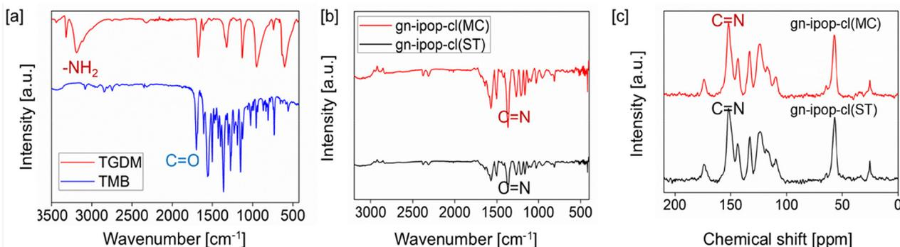
Fig. 1 [a] FT-IR spectra for TGDM, and TMB. [b] FT-IR spectra for gn-ipop-cl. [c] CPMAS <sup>13</sup>C NMR spectra of gn-ipop-cl.
