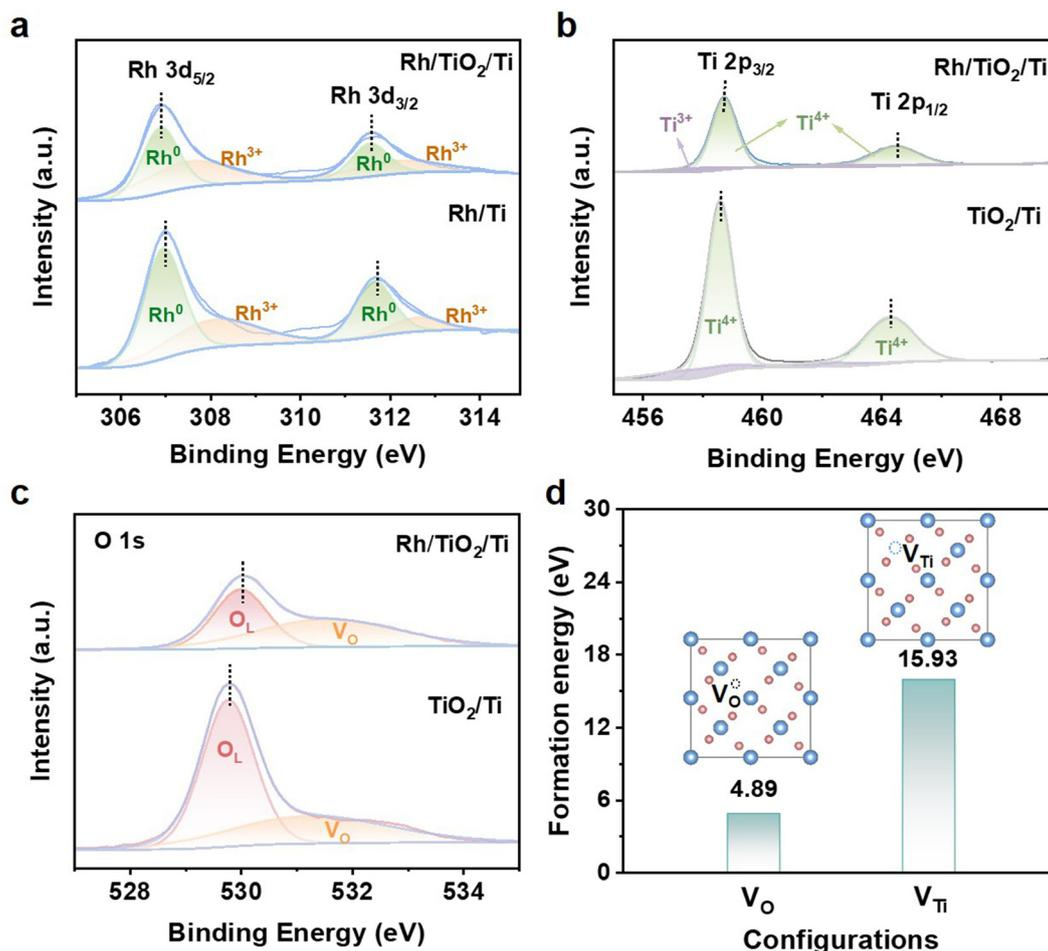
Fig. 3 XPS spectra of Rh/TiO<sub>2</sub>/Ti, TiO<sub>2</sub>/Ti and Rh/Ti. (a) Rh 3d, (b) Ti 2p, and (c) O 1s. (d) Formation energy of V<sub>O</sub> and V<sub>Ti</sub> in Rh/TiO<sub>2</sub>/Ti.
