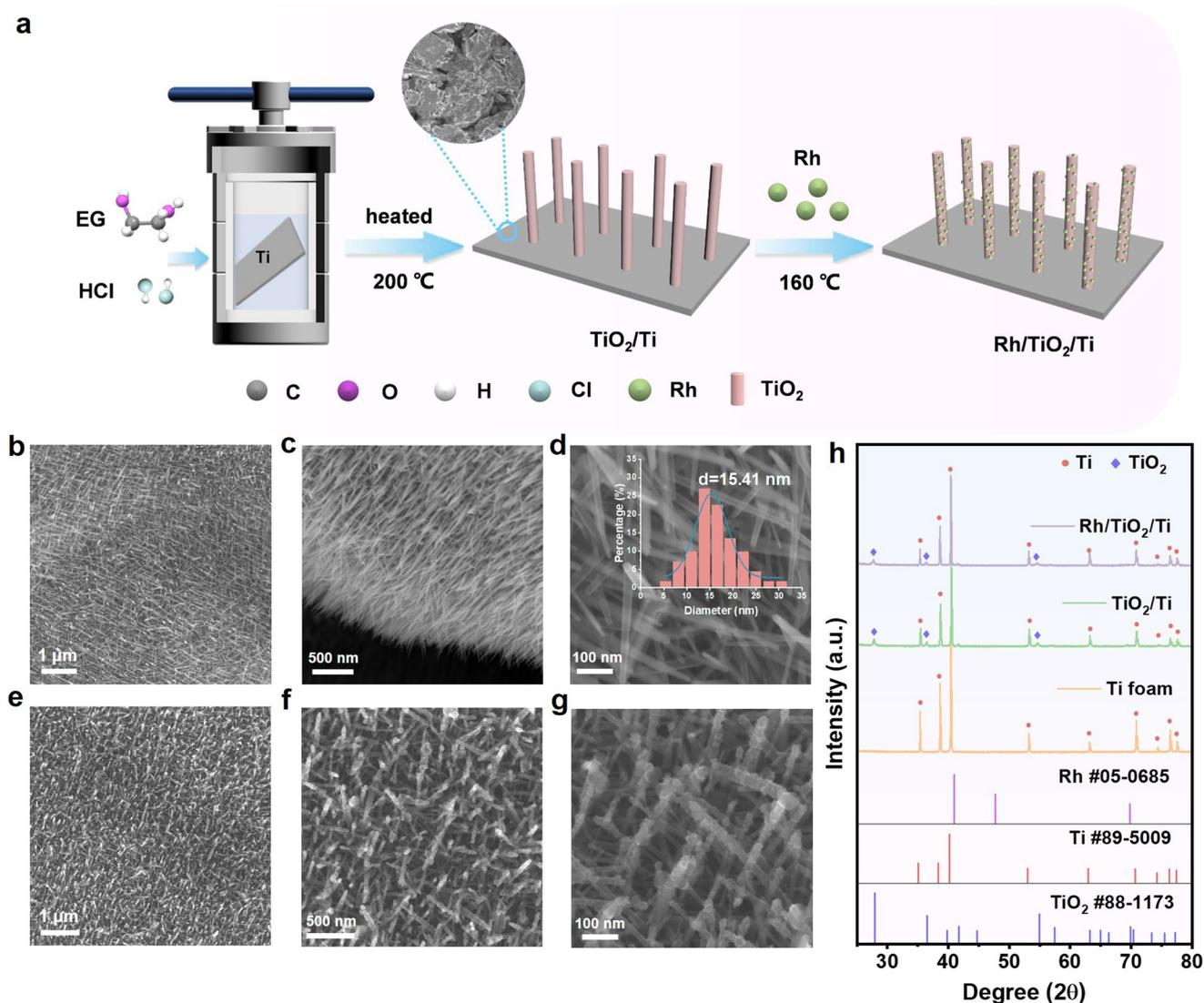
**Fig. 1** (a) Schematic diagram of the preparation process of Rh/TiO<sub>2</sub>/Ti. (b–d) SEM images of TiO<sub>2</sub>/Ti. Inset shows the diameter size distribution diagram. (e–g) SEM images of Rh/TiO<sub>2</sub>/Ti. (h) XRD patterns of Rh/TiO<sub>2</sub>/Ti, TiO<sub>2</sub>/Ti and Ti foam.
