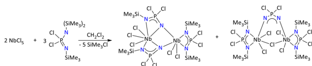
Scheme 25 Synthesis of unusual heterocycles of niobium stabilized by iminophosphoramidate. 91
